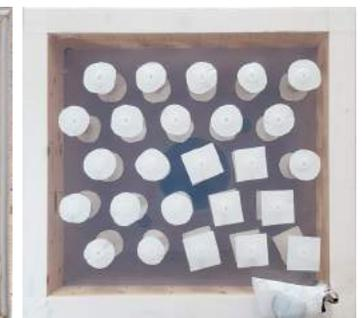
Figure 144: wooden acoustic box with integrated speaker with the panel placed on top
