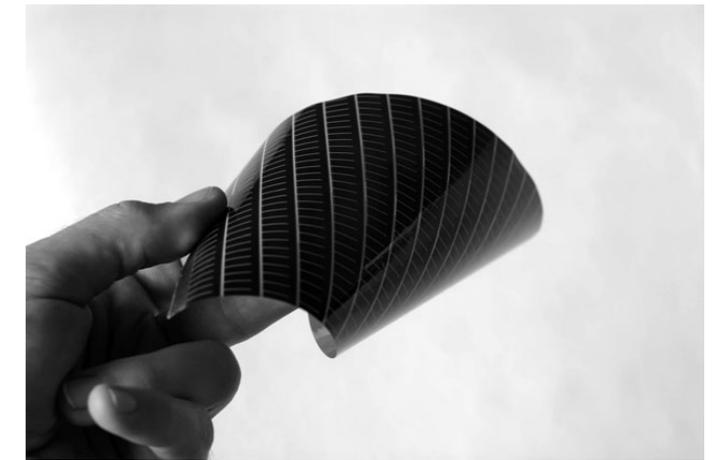
Figure 7: Fully flexible a-Si PV on polymer substrate
