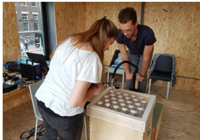
Figure 150: measurement of the panel while deflating it with the hand pump
