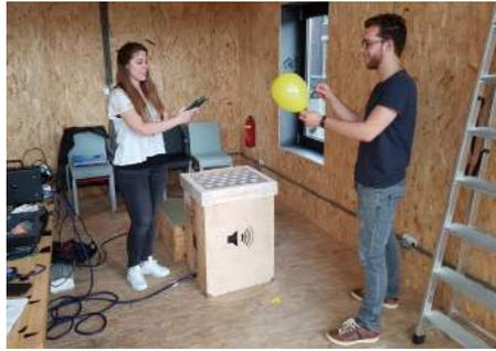
Figure 145: balloons test for measuring the reverberation time
