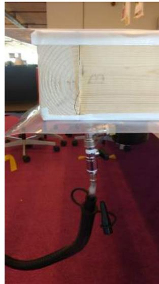
Figure 130: crack in the frame because of vacuum forces
