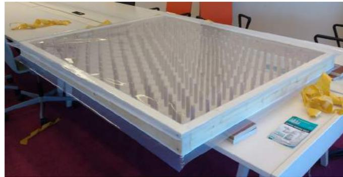
Figure 129: placement of the ETFE in both sides with double-sided tape
