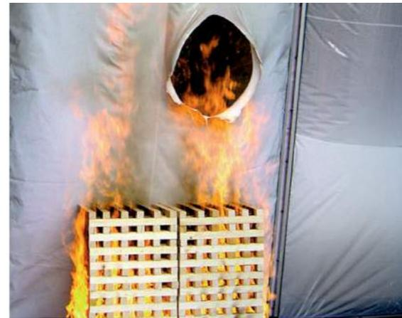
Figure 265: fire test of ETFE (source: Behling, S., Brensing, C., Fuchs, A., Ingenhoven, C., 20101, Innovative Design and Construction, DETAIL, page 49)
