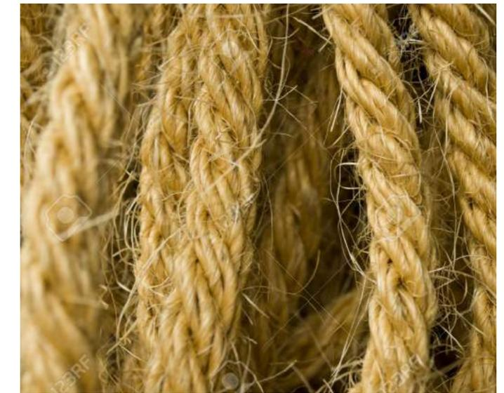
Figure 1: rope made from natural hemp fibres
