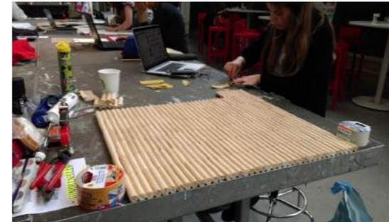
Figure 123: cutting and sanding of the spacers
