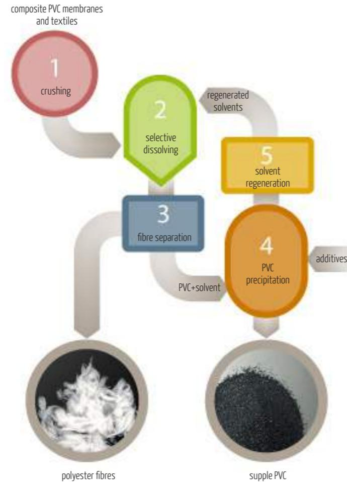
Figure 20: Separation of the components of the flexible composite materials in order to create single raw materials
