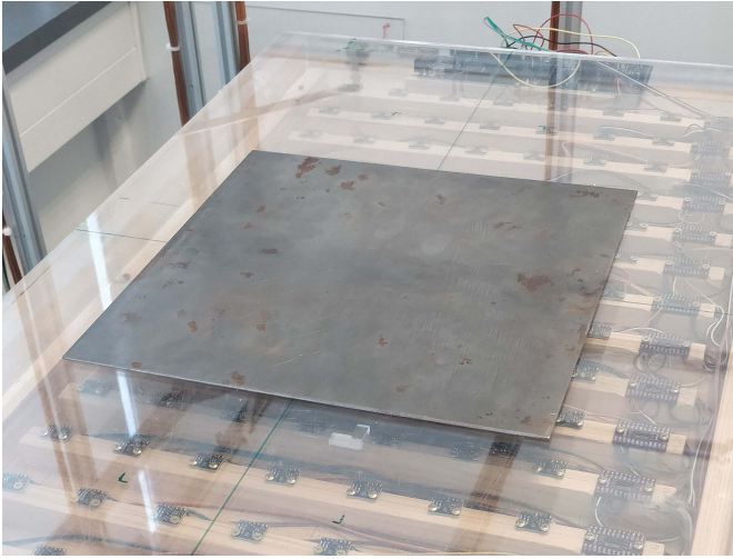
Fig. 6. Steel plate above sensor array.
