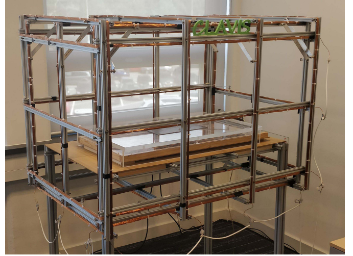
Fig. 4. Measurement facility “CLAViS” that contains a coil configuration to change the ambient field in three directions.
