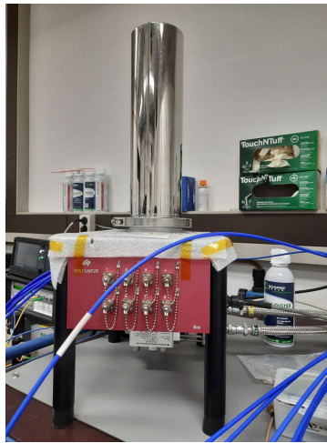
Figure 12: Picture of the cryostat used in this experiment. The SNSPD is mounted inside. The slots (eight) are also visible. The rest of the setup is the same as in figure 8.
