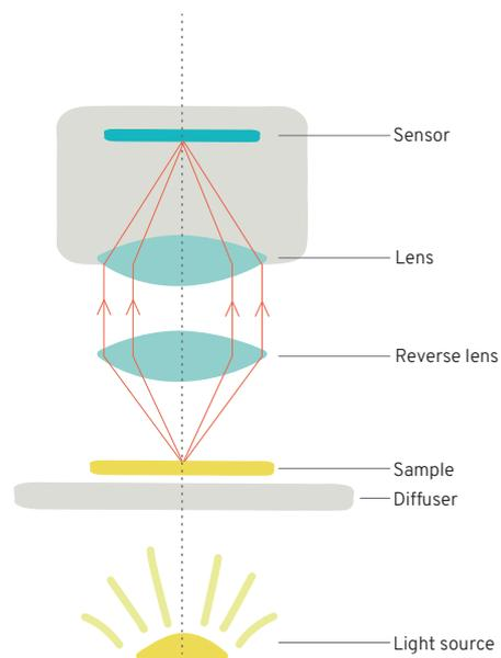
Figure 6. Set up of Schistoscope
