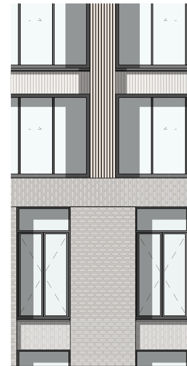
10. Façade cladding is applied on site: brickwork, prefab lintels and timber slats.
