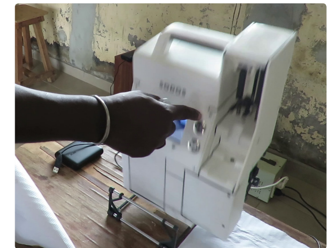
Figure 56. Integrated prototype as it is falling from its stand during a user test in Ivory Coast.
