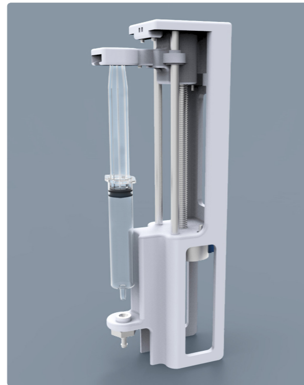
Figure 18. The digital design of the initial fluid insertion system.
