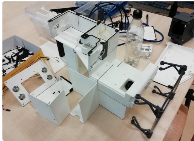
Figure 40. The partially assembled 3D-printed parts of the integrated prototype.
