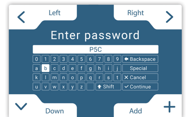
Figure 35. Improved interface with virtual keyboard for entering Wi-Fi passwords shown on scale 1:1.
