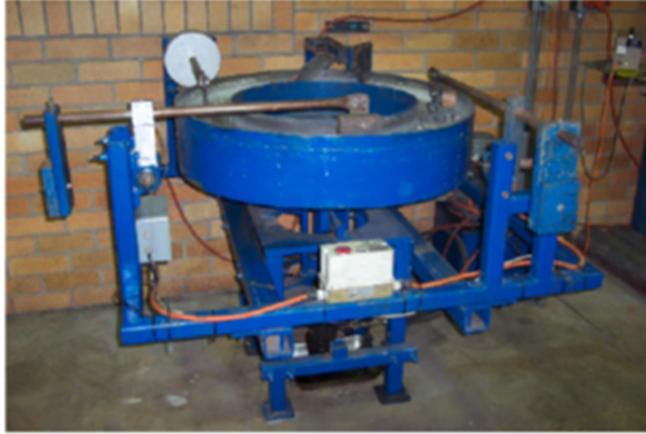
Figure 2.23: Circle bed wear tester [72] (picture provided by G. Lodewijks)
