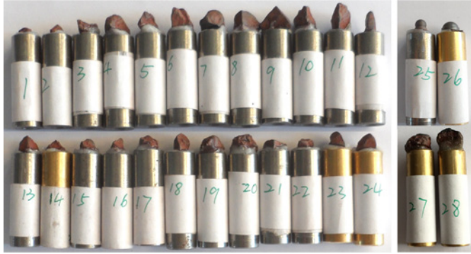
Figure 4.9: Experimental pins with SiShen particles
