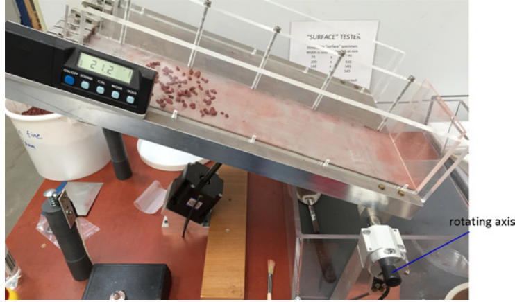
Figure 4.28: Measuring the coefficient of static friction of discrete particles
