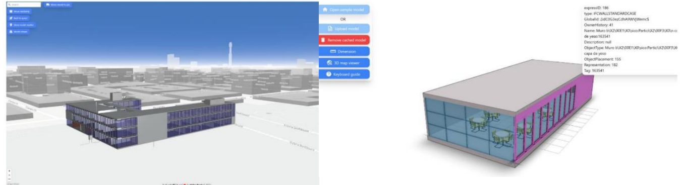
Place BIM model everywhere in Mapbox, reading IFC properties by clicking elements before placing. (Helenkwok, 2023)
