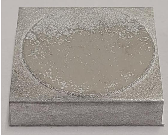
ASTM C633 minimum thickness (0.38 mm)
