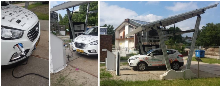
Figure 2-1 Experimental Fuel Cell Electric Vehicle-to-Grid (FCEV2G) set-up at The Green Village, Delft University of Technology, Delft, The Netherlands.
