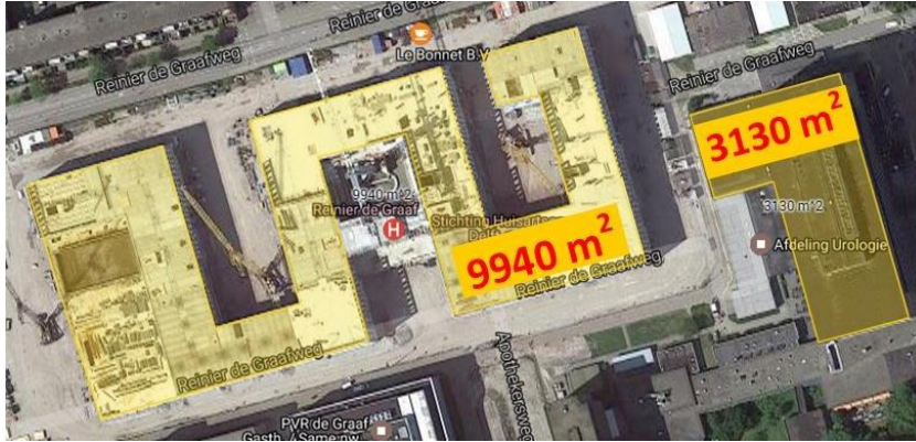
Figure 4-2 Reinier de Graaf Gasthuis hospital and its car parking area with a total potential surface area of 13,070 m 2 to place solar panels.
