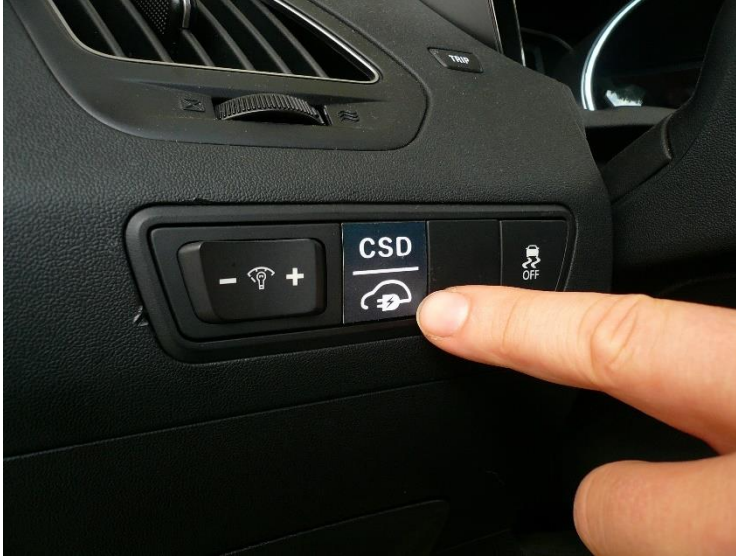
Figure 2-4 New dashboard V2G activation button also initiates Cold Shut Down.
