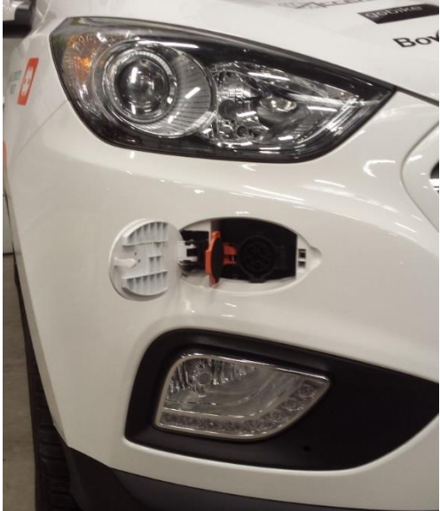
Figure 2-3 V2G Type 1 Socket integrated in the front bumper.
