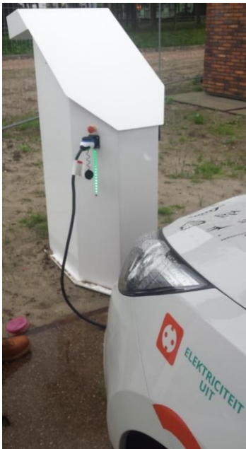
Figure 2-5 V2G-DCAC unit connected to the FCEV.
