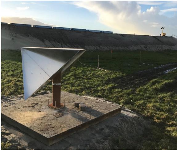
**Figure A.5:** The reference corner reflector [167] installed on a Stelcon plate, on top of an extra layer of sand.
