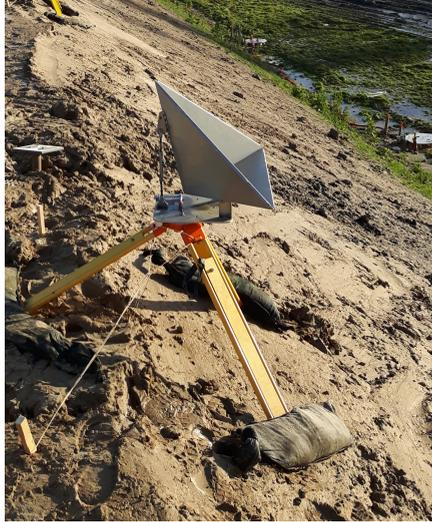
**Figure A.1:** The design of corner reflectors for Eemdijk.
