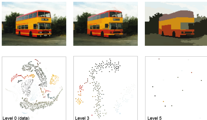
Figure 6.2. RGB image (top left) and 2 levels of abstraction (3 and 5). Superpixels are recolored with the average color of all pixels they contain. Numbers of components: 15300 (150x102 pixels), 271, 14.
