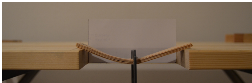
Multiple direction birch - Max load of 40.21 N
