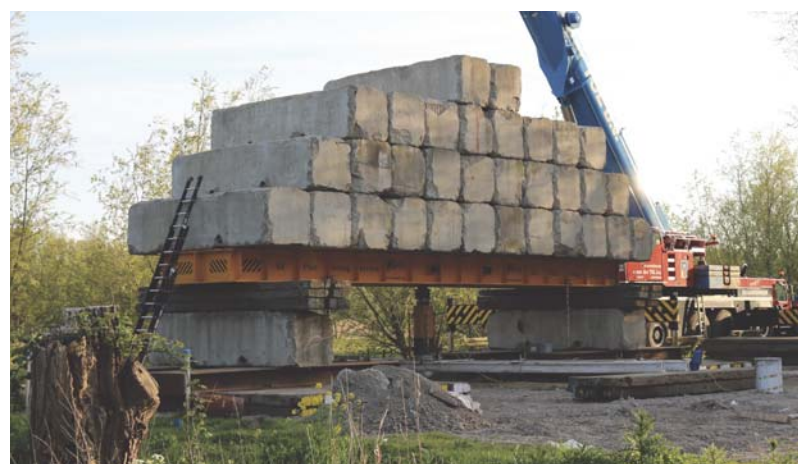
Figure 1 – Testing screw injection piles at Delft with a load test frame and concrete ballast.
