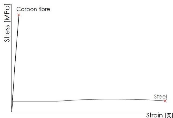
Figure 3.1: Stress-strain curves carbon fibre and construction steel
