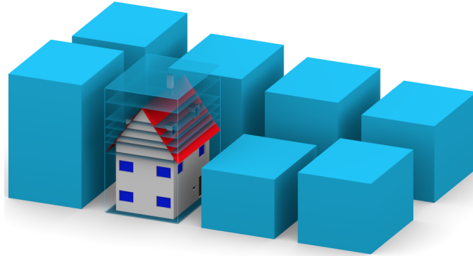
Figure 2.1: Seven different roof height references for a single building (in LOD3) [Biljecki et al., 2014].
