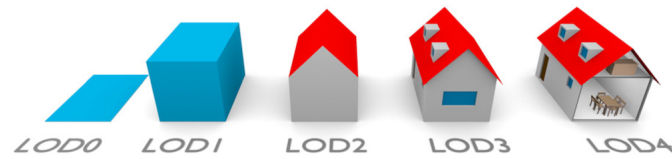
Figure 1.2: The five LODs as specified by the OGC for CityGML version 2.0 [Biljecki et al., 2016a].
