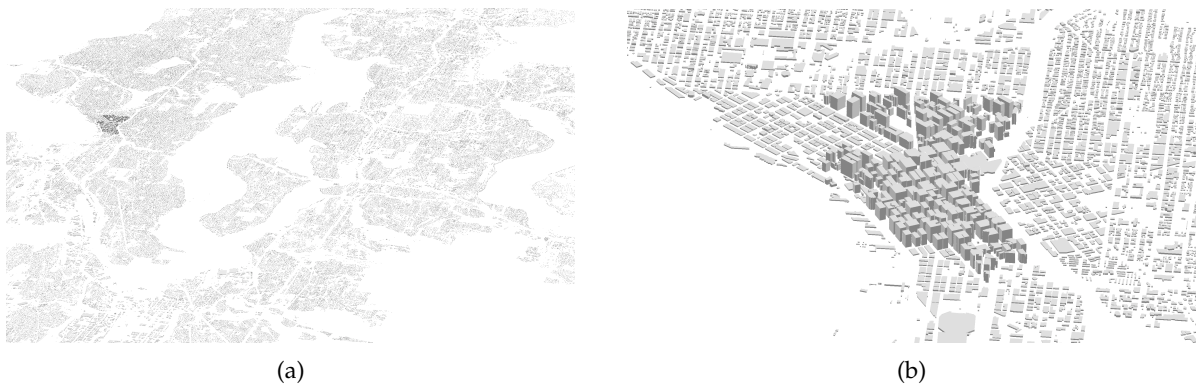
Figure 5.1: 3D city model of the results for Seattle, Washington, using the height predictions from the RFR method. The prediction model is trained on only the suburban and rural training data. (a) provides a general overview, while (b) shows a close-up of the CBD.
