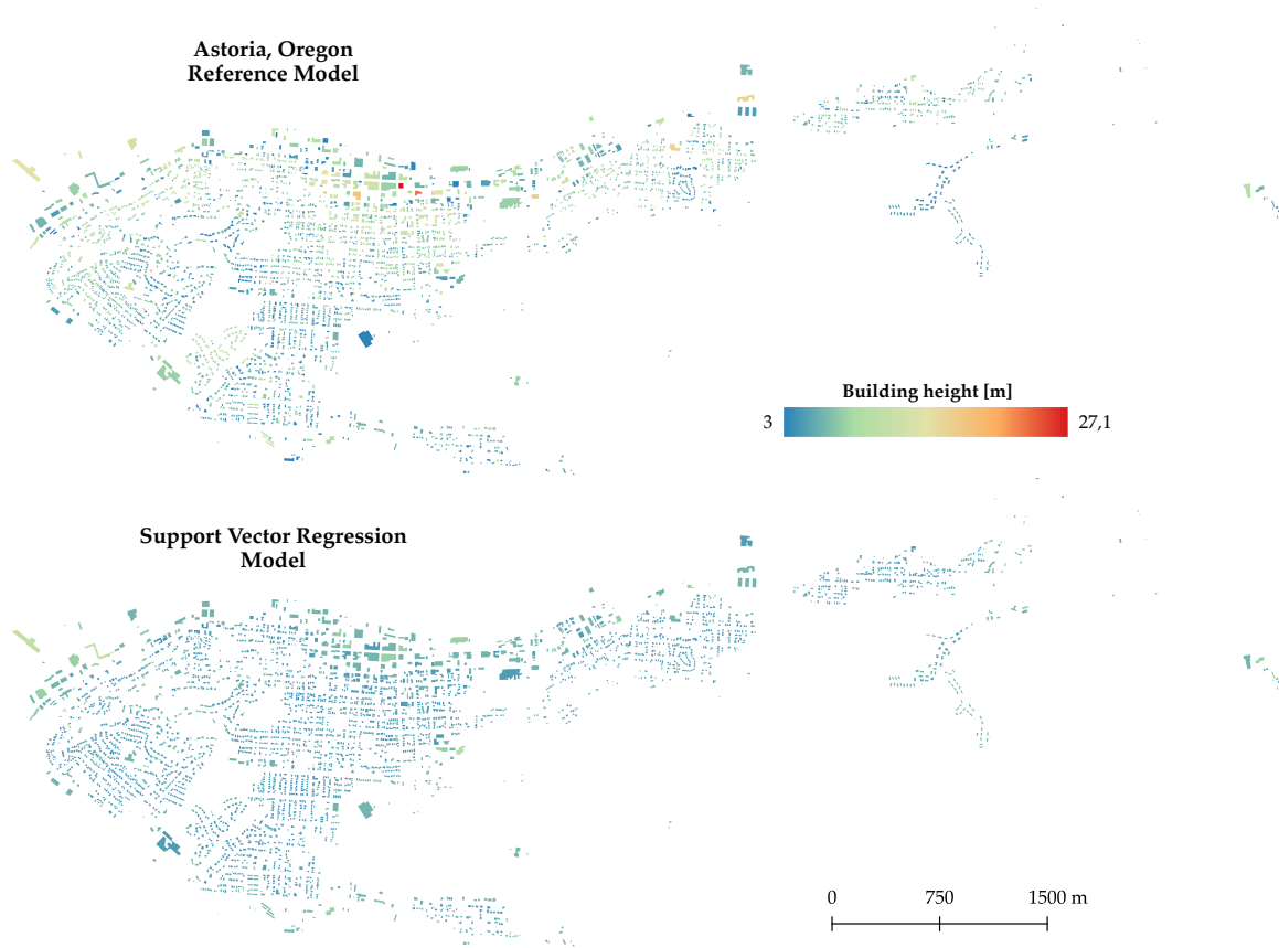
Figure D.9: Maps showing a comparison between the building heights in the reference model and the SVR building height predictions for the town of Astoria, Oregon. The prediction SVR model is trained on only the rural and suburban data.
