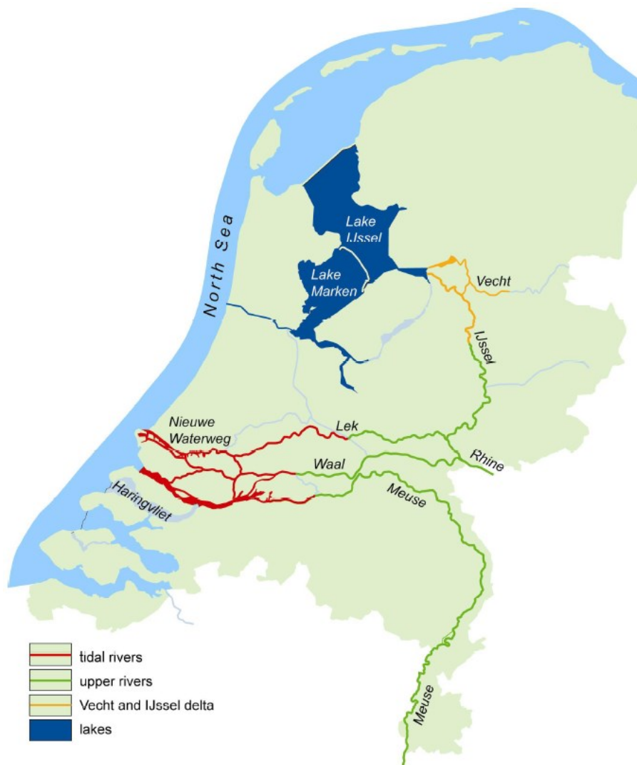
Figure 4: Sub-systems of the water system of The Netherlands (Geerse, 2011)
