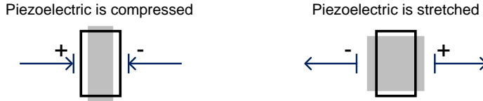
Fig. 2.6: Piezoelectric phenomenon during compression and stretching [56].
