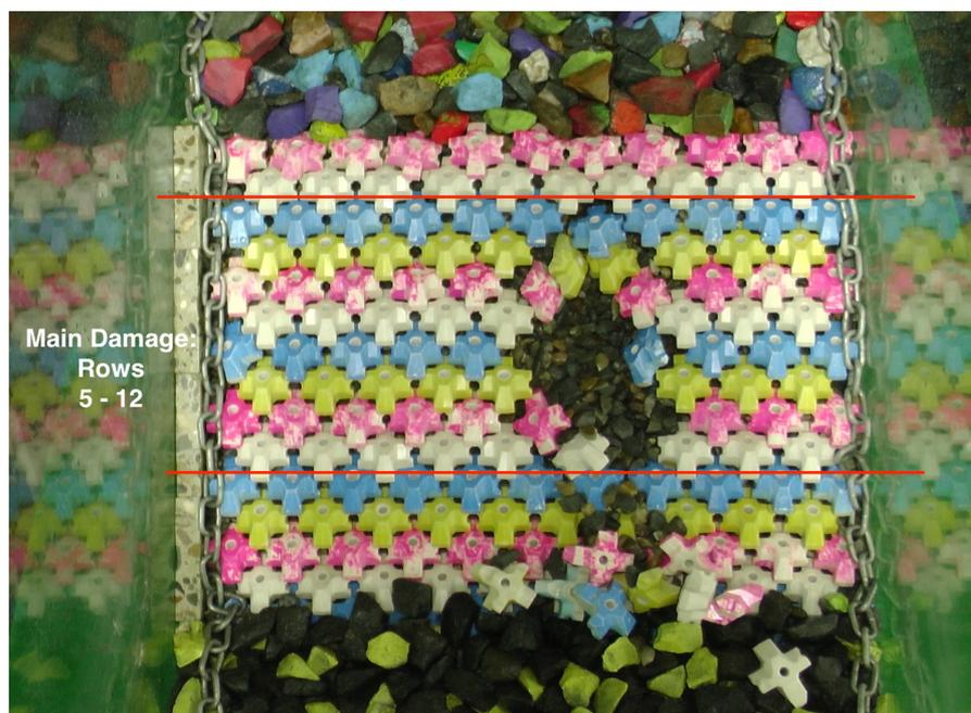
Figure 4.25: Damaged area occurred during Series 3.
