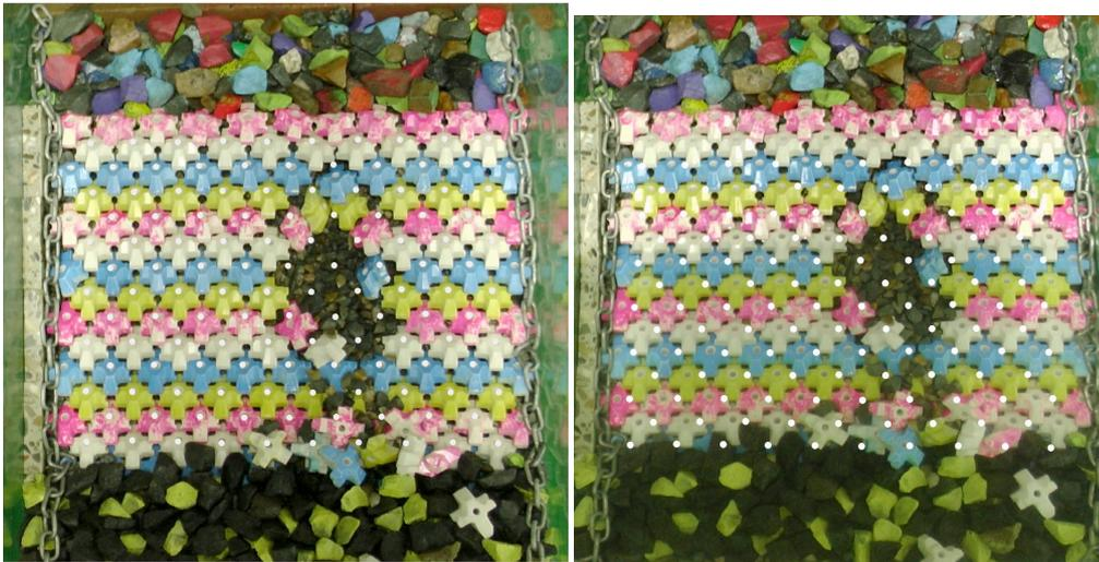
Figure D.3: Displacement of armor layer units during tests from Series3.
