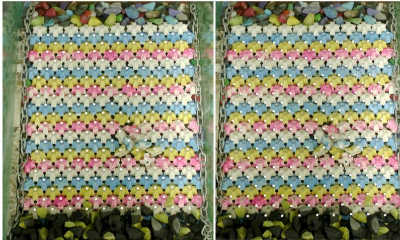
Figure D.5: Displacement of armor layer units during tests from Series5.
