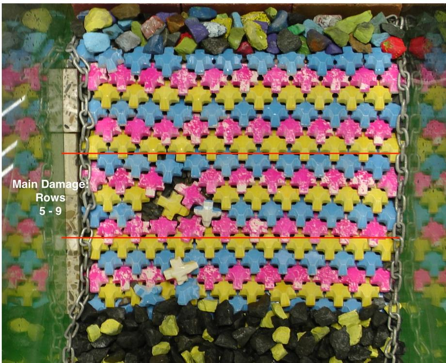
Figure E.1: Damaged area of armor layer units during tests from Series1.
