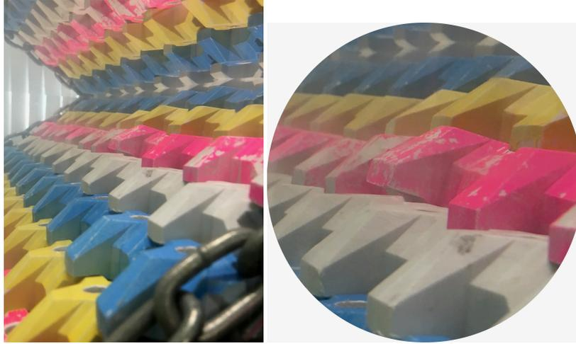
Figure 4.6: Xbloc+ slightly rotated backwards.
