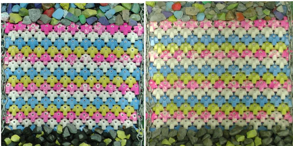
Figure 4.21: Placement of armor layer during series 3.
