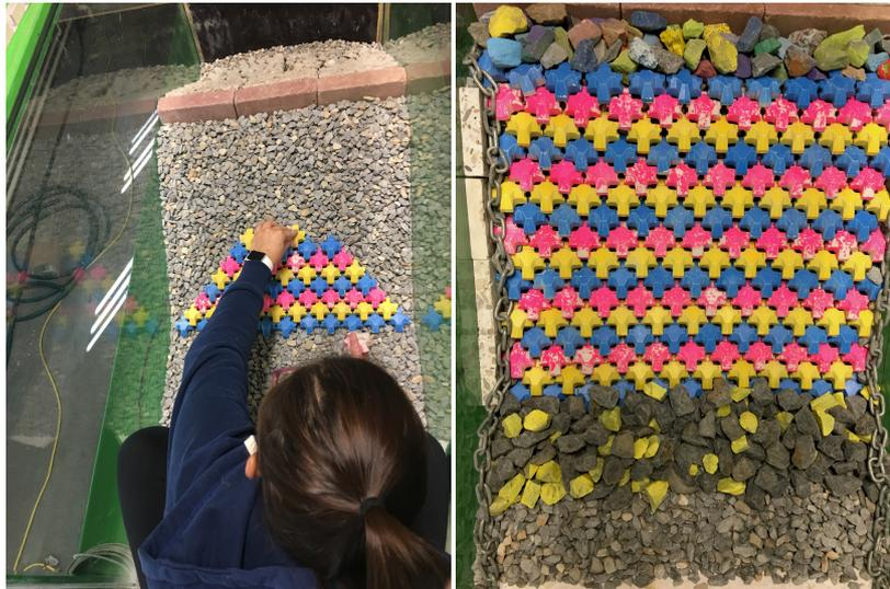
Figure 3.3: Placement of armor units
