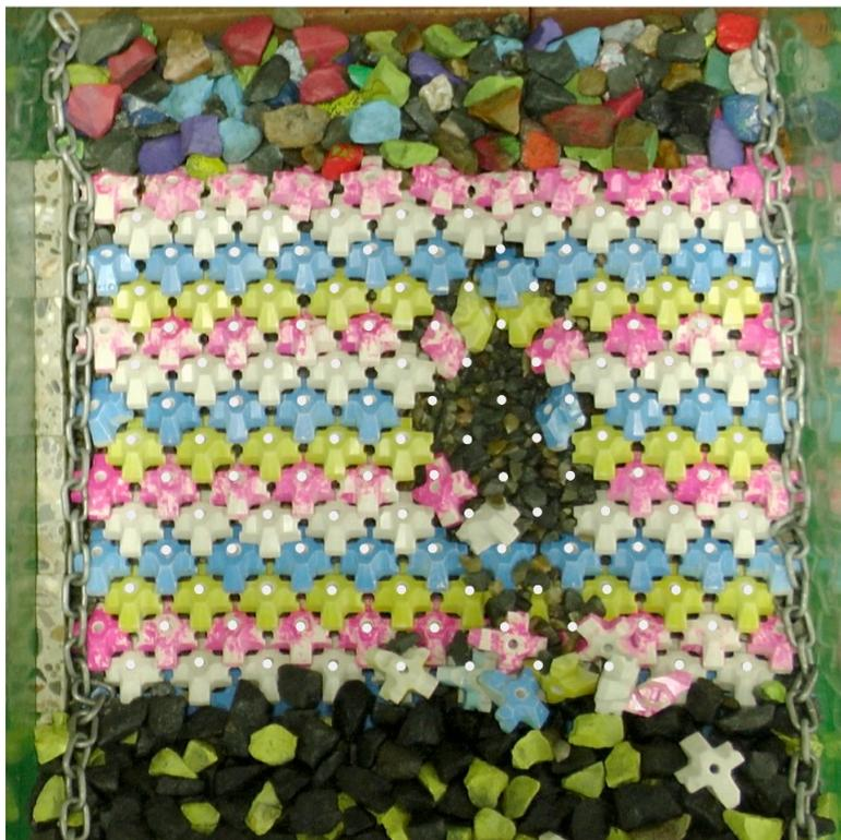
Figure 4.13: Displacement of units occurred during Series 3.
