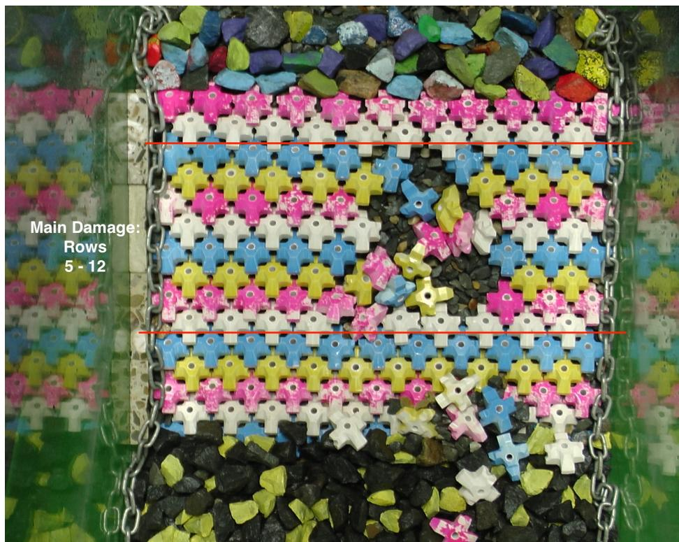
Figure E.3: Damaged area of armor layer units during tests from Series4.
