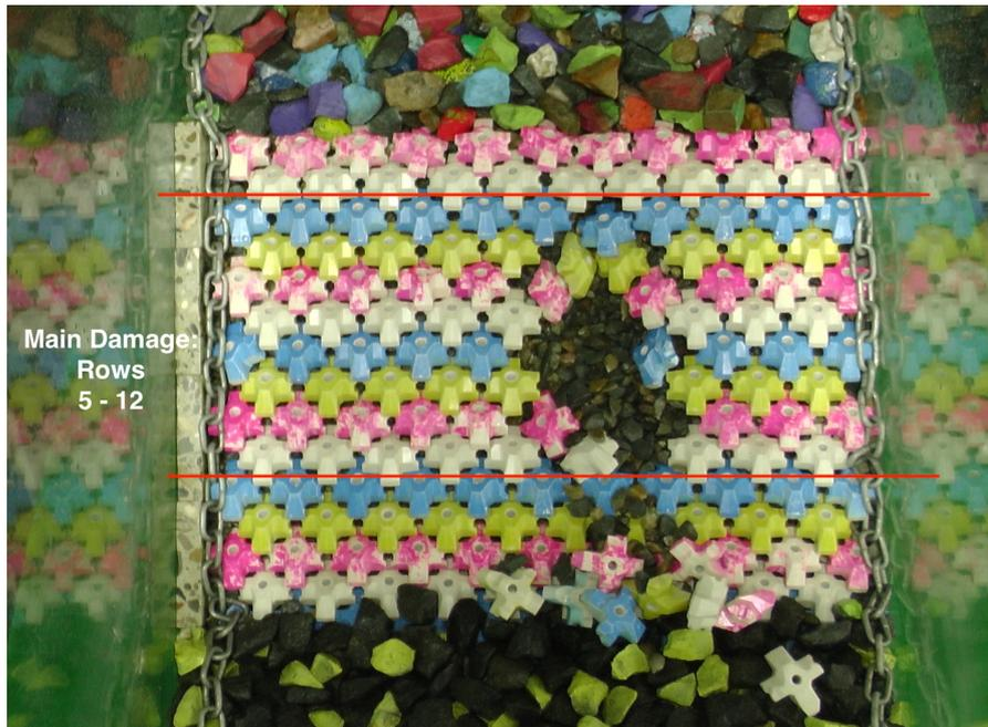
Figure E.2: Damaged area of armor layer units during tests from Series3.
