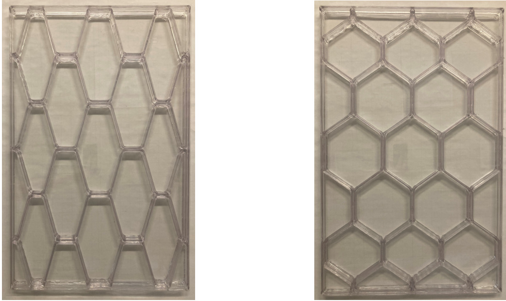
(a) The finished panel with hexagons in horizontal direction. (b) The finished panel with hexagons in vertical direction.
