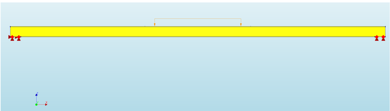
Figure 310: Side view of the geometry of the model with the load, supports, and boundary interface elements.
