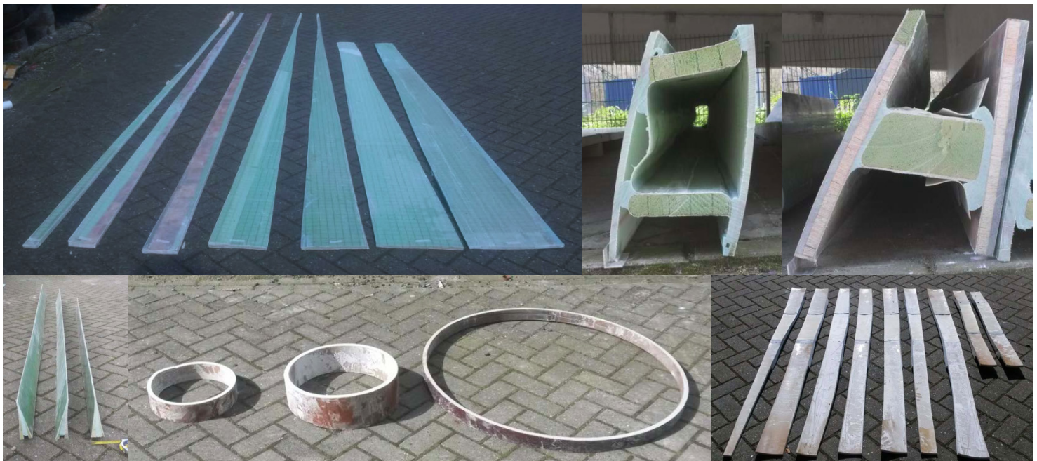
Figure 24: Construction elements cut from a rotor blade (ten Busschen et al., 2016)
