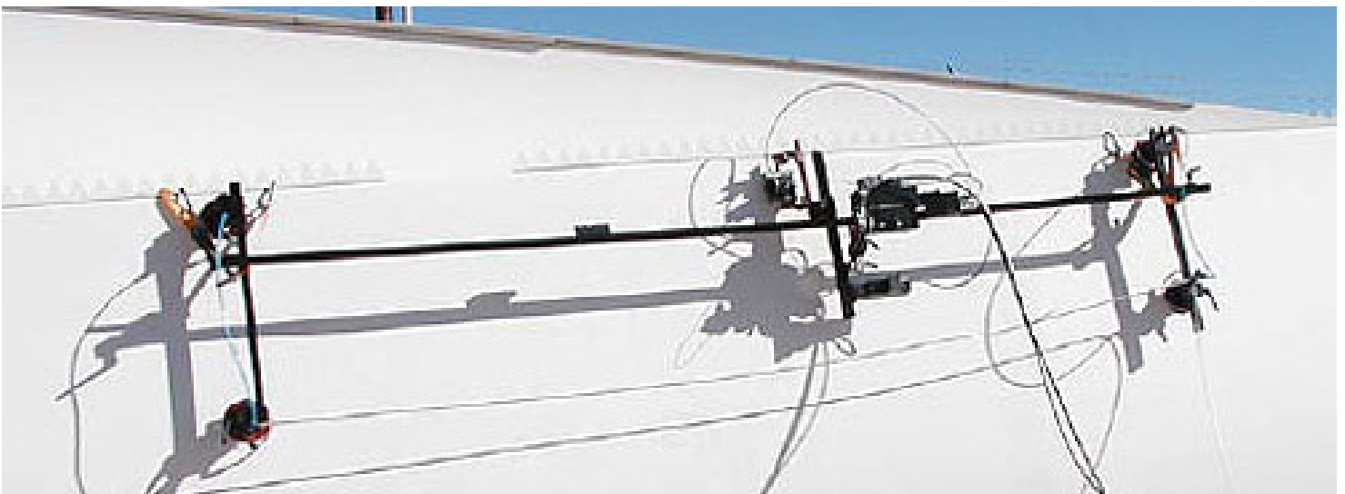
Figure 58: Ultrasonic blade inspection
