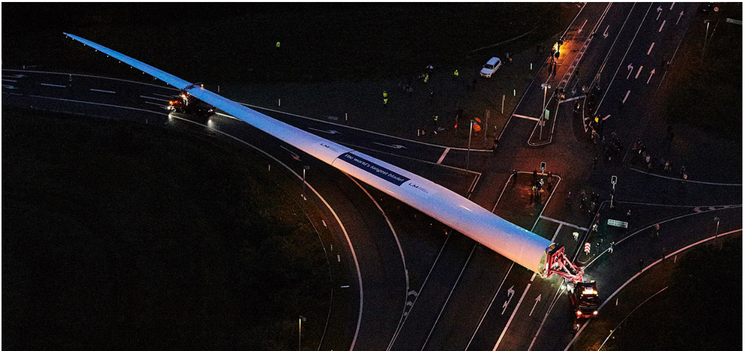
Figure 59: Transporting the world's longest blade
