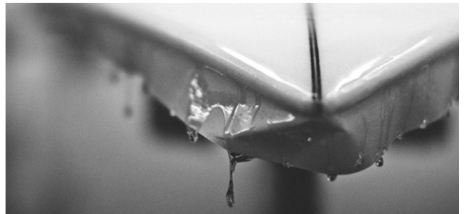
Figure 6: In a surfboard construction, a fiberglass (dispersed phase) and epoxy/polyester resin (matrix) composite shell is wrapped around an EPS/PU foam core (sandwich). Most surfboards also have a wooden 'stringer' glued into the foam construction for extra strength and stiffness.
