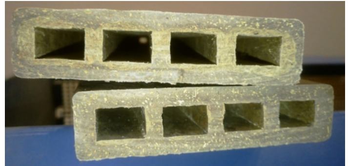
Figure 25: (bottom) Hollow decking boards (Conenor, n.d.)
