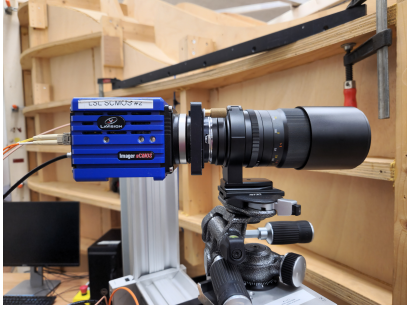
Figure 3.13: LaVision Imager sCMOS camera.
