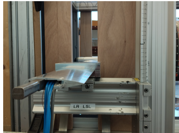
(b) X-beam mount showing vertical scale and sting mechanism.
