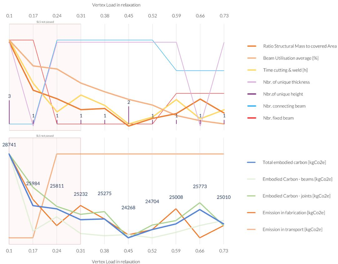
Figure 5-9 Normalized objectives data output from design exploration (top to bottom a, b)
