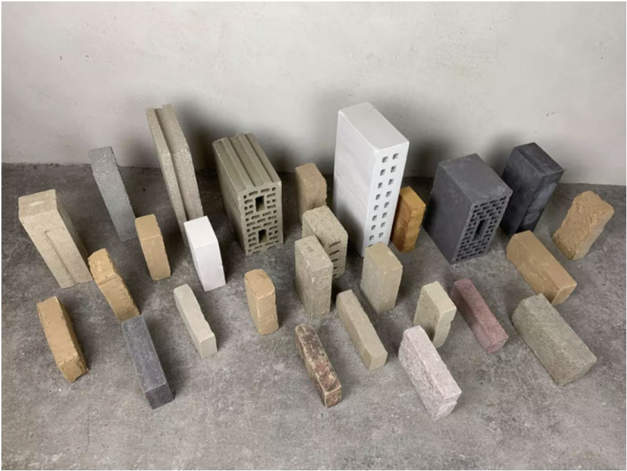
“Utube”: Clay bricks from Metro3 excavation, Bruxelles ,2021 [BC Materials]
