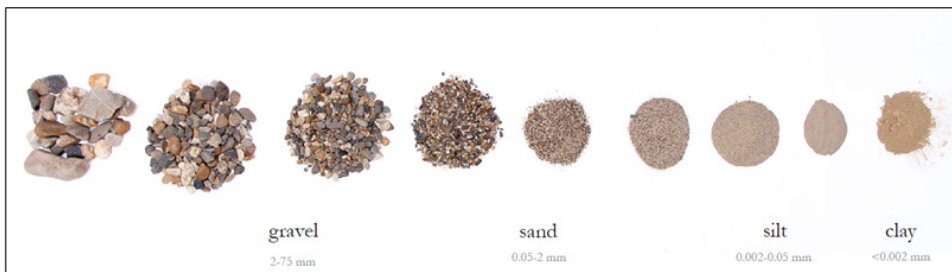
Fig. 15. Resources and particle size of Geobased Building Materials [BC Materials]
