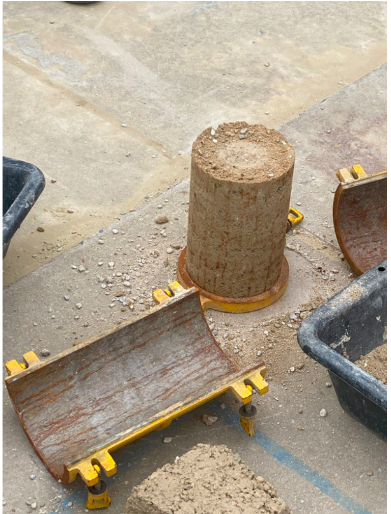
Fig.1. Visit to BC Materials for Earth Discovery Day, compression test for Rammed Earth in steel mould [Workshop] 2024. Author
