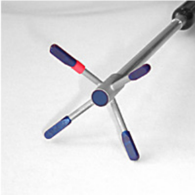
Figure 3.4: Detail of the ADV probe
