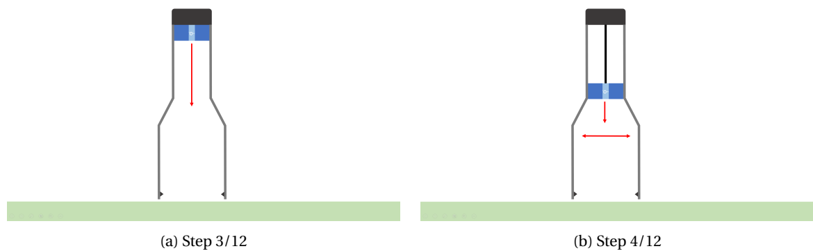
Figure 3.2: Installation procedure of a monopile (step 3+4)
