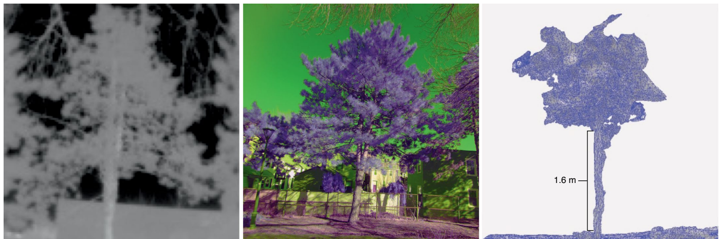
Fig. 2 | Examples of three imaging-based methods used to estimate urban greenery health attributes. From left to right: a thermal image captured using a longwave-infrared (at 8–14 \mu ) FLIR Lepton 3.5 camera, a multispectral image
