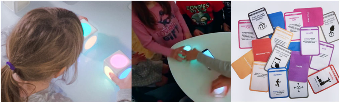
Figure 1: Left: Lumies are connected toy blocks that can respond to touch, orientation, acceleration, proximity to other blocks – and respond with colored lights, sound and vibration. They are digital playthings that can be played individually or socially—with or without a phone screen (middle). The possibilities seem endless—and yet hard to imagine. To help experts and children consider gameplay possibilities, we designed a card deck for exploring the gameplay design space (right).
