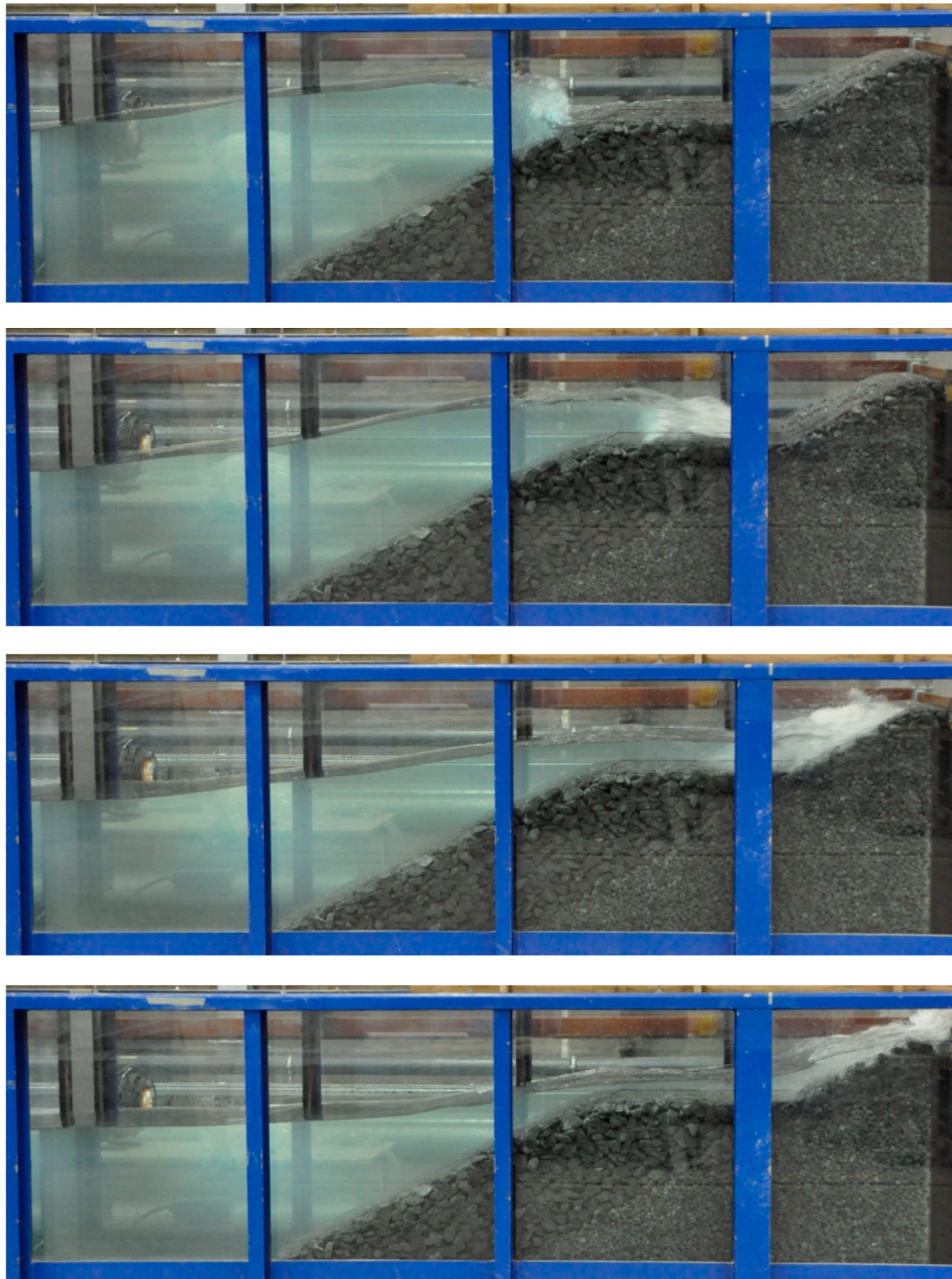
Fig. 6. Pictures of waves on a rubble mound breakwater with a berm and a crest wall (Configuration 4; B = 0.75 m, R_c = 0.3 m, H_{m0} = 0.224 m, s_{m-1,0} = 0.023 ).
