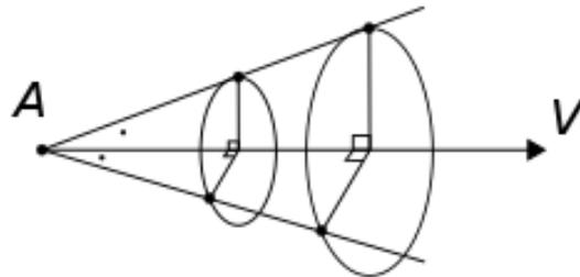
Figure 1: Aircraft A and four points with the same angle between distance and velocity vector forming a cone
