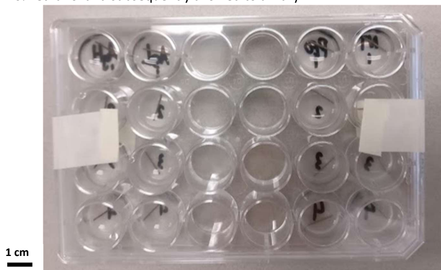
Figure 10. Static bacterial adherence in 24 wells plate (n = 4 implants per group).
