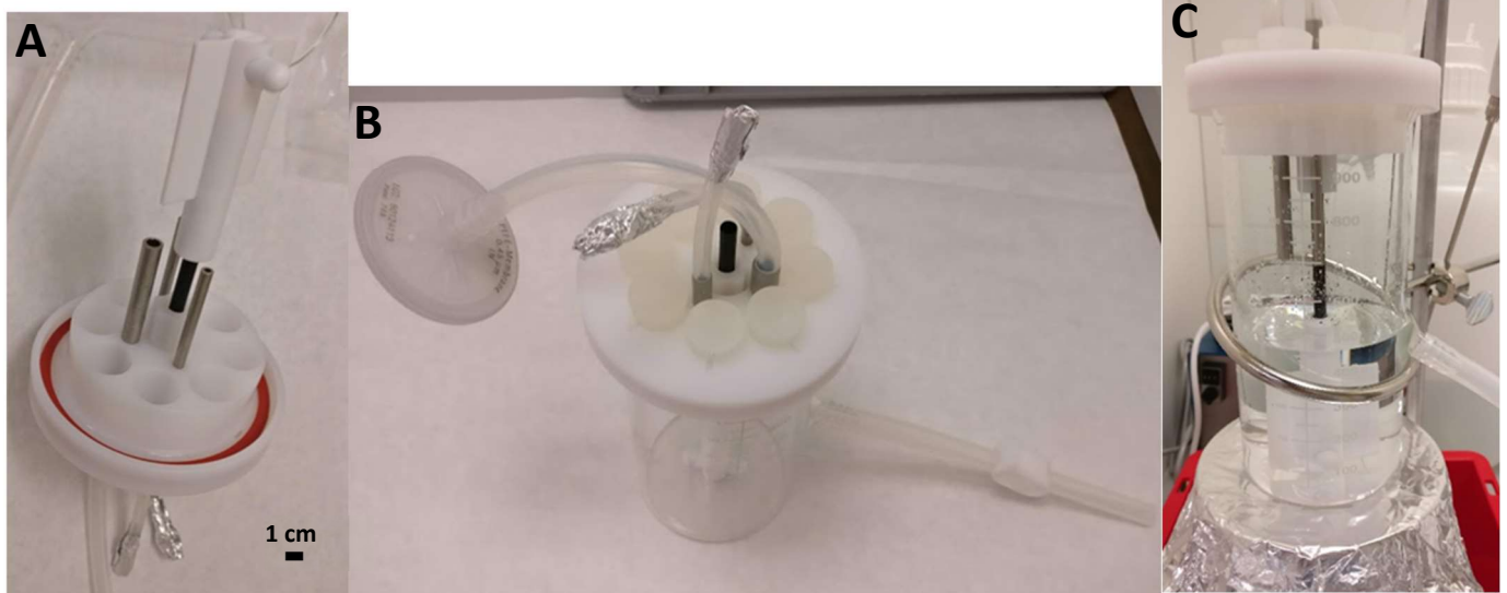
Figure 8. Assembly of the reactor. (A) Lid and stir mechanism. (B) Reactor and waste tubing. (C) Placement on top of stir plate.
