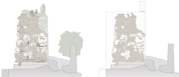
Figure 22. Drawings showing the original fragments and the volumetric restoration of the tower.
