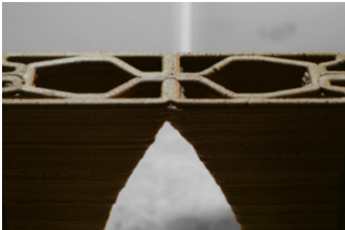
Figure 41. Variable infill density in printed object.
