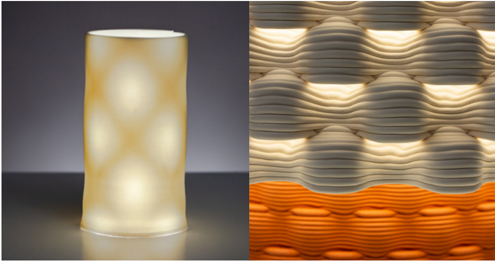
Figure 34. Light diffusion through extrusion variability (left) and through toolpath variability (right).
