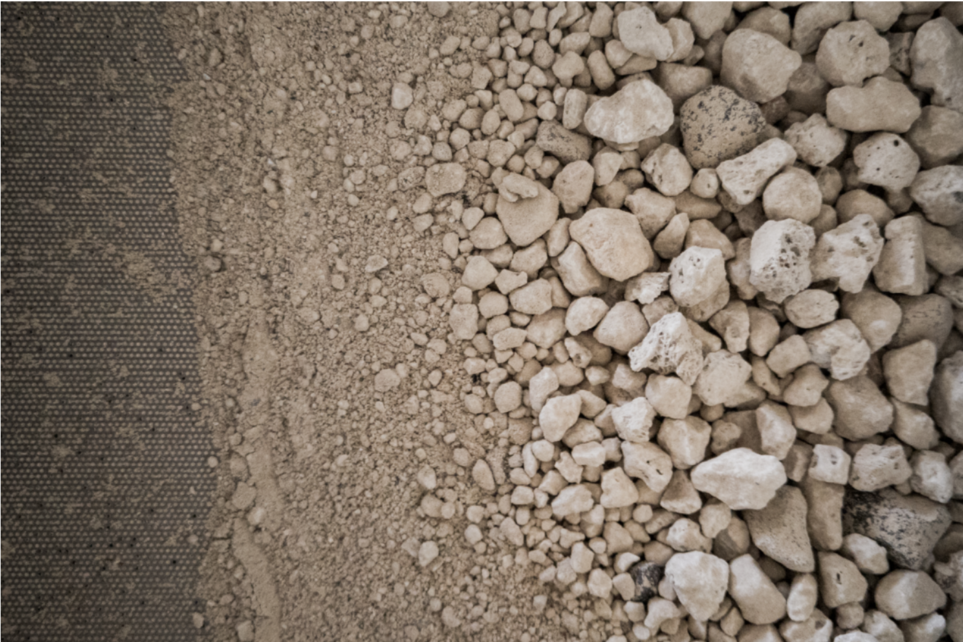
Figure 163. Sifting of Theran earth through a 1mm sieve.
