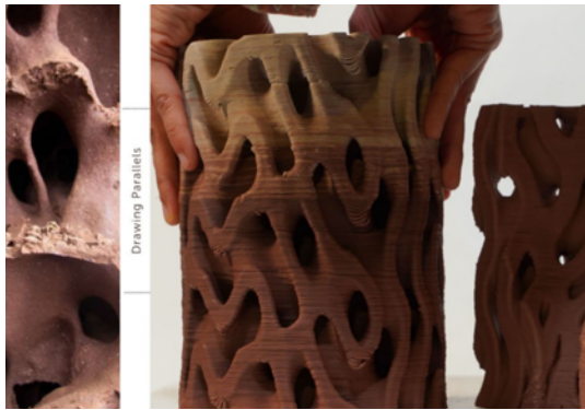
Figure 59. Biomimetic inspiration on termite mounds for airflow.
