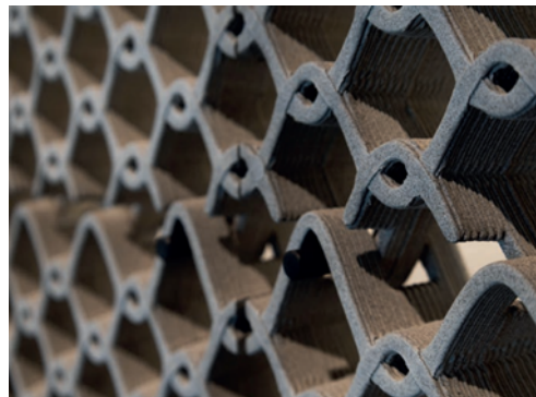
Figure 77. Print detail showing overlapping printing paths.
