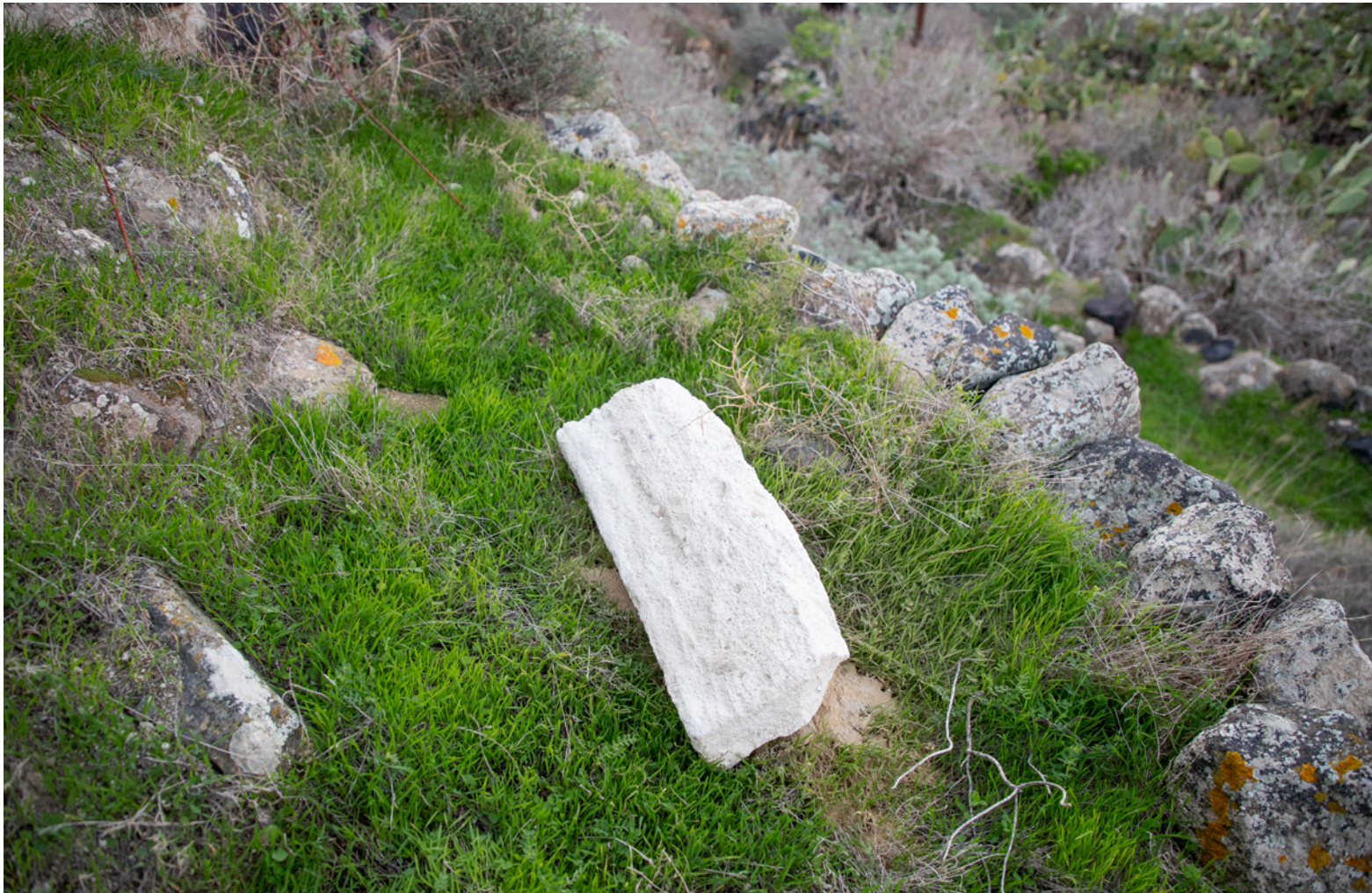
Figure 127. Rectangular brick made of Theran mortar with pumice stone aggregates
