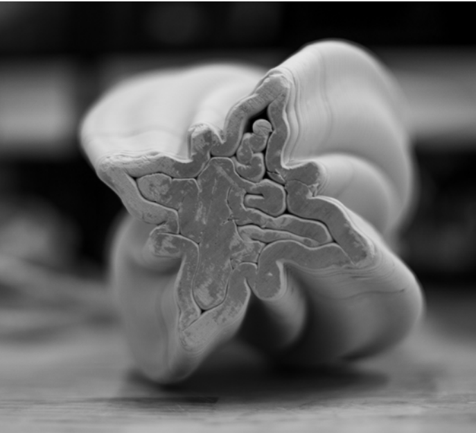
Figure 145. Effect of infill printing bottom caps in an LDM 3D-printed object.
