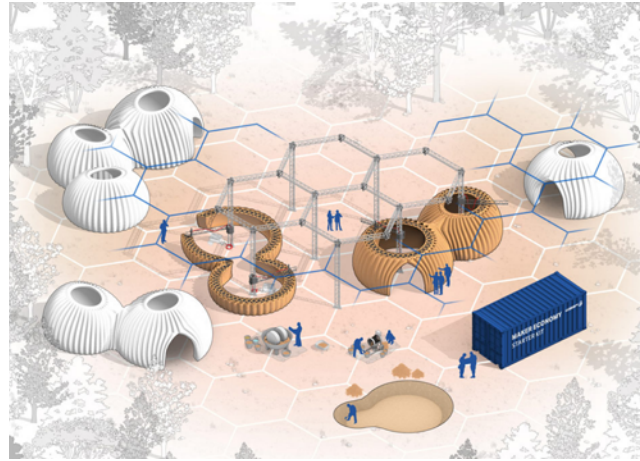
Figure 70. WASP's "Maker economy starter kit", an LSAM system that includes material sourcing, processing, and printing facilities all in one place.
