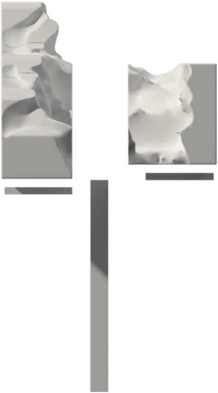
Figure 152. Splitting of the lintel into inside and outside tiles for an easier integration of the non-printed elements (side view).
