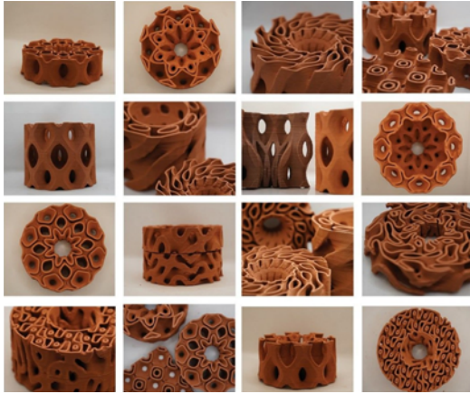
Figure 58. Infill geometries optimized for air flow.
