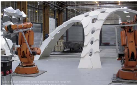
FIG. 21 Prototype developed by means of robotic fabrication implemented with two large ABB robots operating wire-cutting tools [2012]
