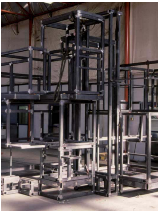
FIG. 39 Steel skeletons of 18 cubical volumes, provisionally bolted together
