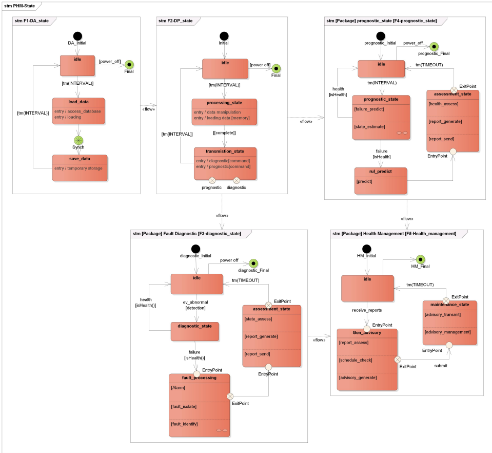
Figure 3.11: Functions operation states of PHM system
