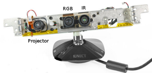
Figure 9-1: The Kinect sensor with its cover removed. From left to right: the infrared projector, the RGB camera and the IR camera. The IR projector and camera are approximately 7.5 centimetres apart. Source: iFixit 2
