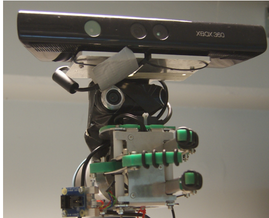
Figure 1-1: The Kinect sensor (top) and a Logitech camera taped to the end effector of the UR5 robot arm. Below it a Fetch Hand from Lacquey.
