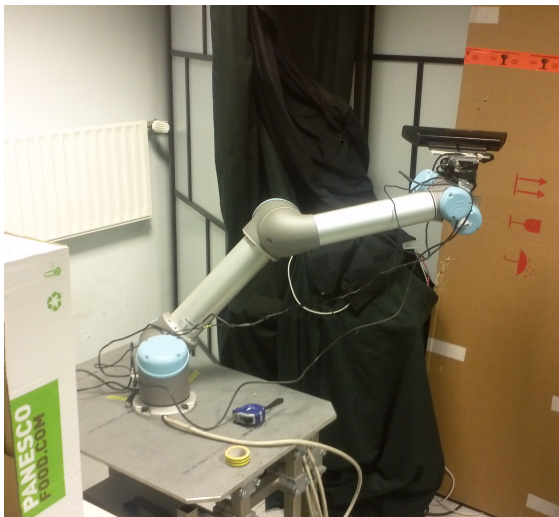
Figure 11-9: Example of the NBV controller making the robot look to the space behind the movable screens.
