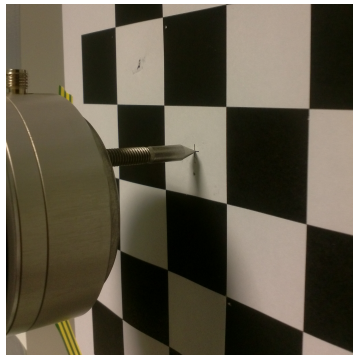
Figure 8-6: The TCP of the UR5 with a bolt fitted in the top left corner thread. The tip of the bolt is pointed at the centre of the checkerboard. The positions of crossings of the checkers are also measured in this way.
