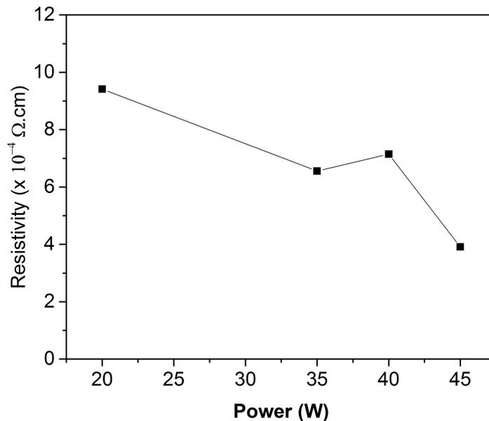
Figure 4.4: ITO resistivity vs deposition power.
