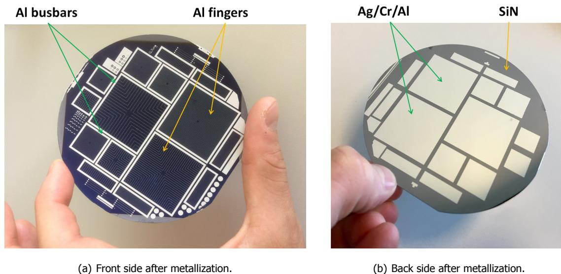
Figure 2.3: Front and back sides of solar cells after metallization.
