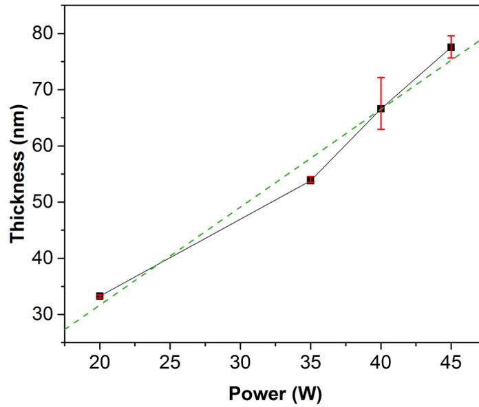
(a) ITO thickness vs deposition power.
