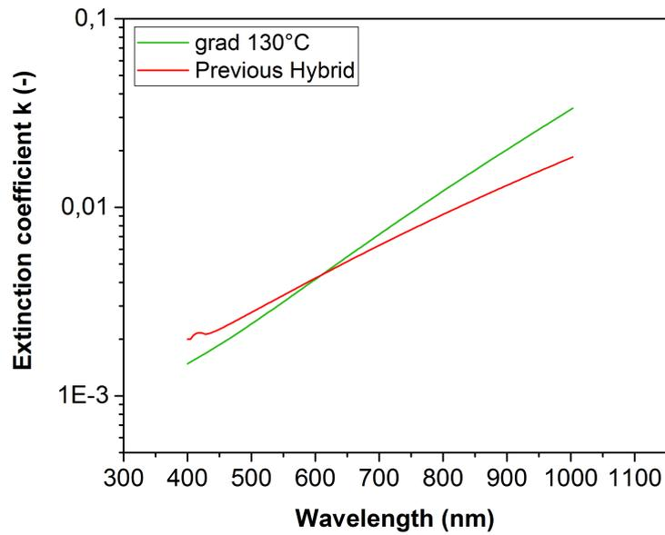
Figure 4.12: Logarithm of ITO extinction coefficient  $k$  vs wavelength.
