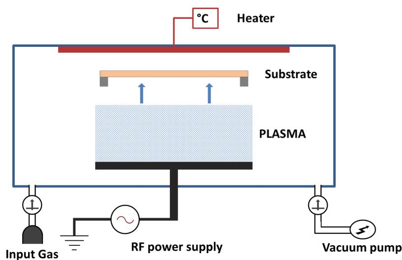
Figure 4.1: Principle of ITO sputtering [29].
