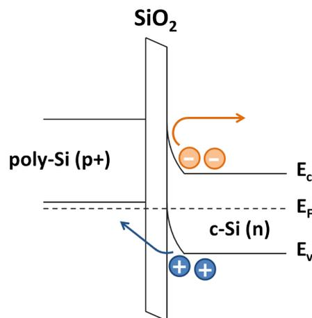
Figure 1.10: Tunnel effect introduced by a  $\text{SiO}_2$  layer at a p-contact interface.
