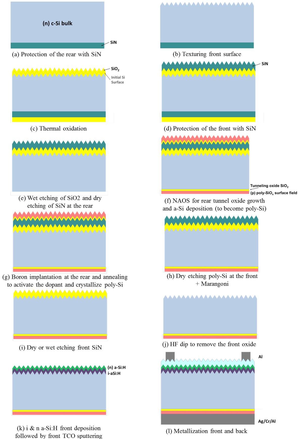
Figure 3.9: Possible flowchart for Hybrid solar cells fabrication with additional oxidation/etching steps.
