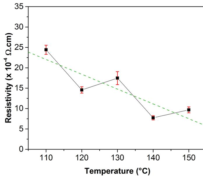
Figure 4.5: ITO resistivity vs deposition temperature.
