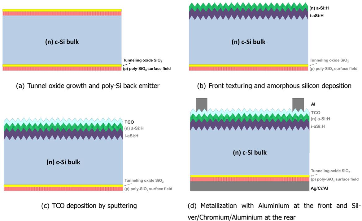
Figure 2.1: General process of fabrication of hybrid solar cells.
