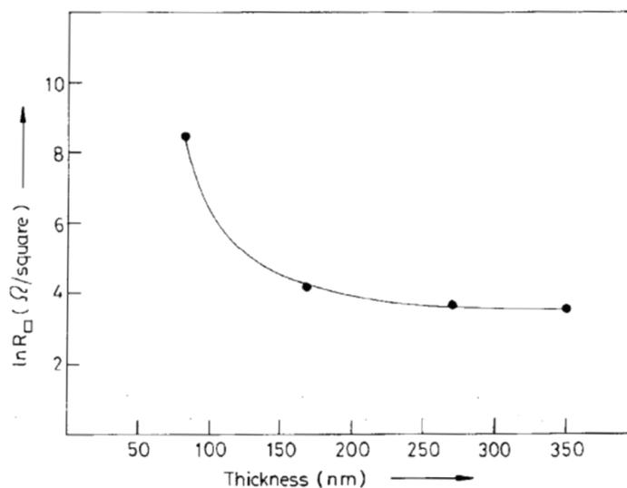
Figure 4.2: Variation of sheet resistance with the ITO thickness [30].
