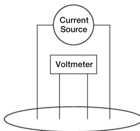
Figure 2.5: Four-Point Probe Resistivity Configuration [23].
