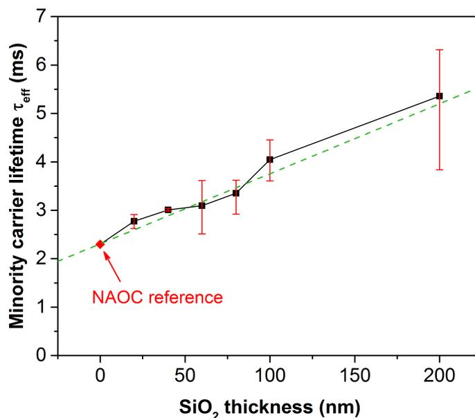
Figure 3.3: Minority carrier lifetime vs oxide thickness.
