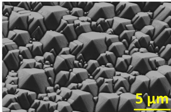
Figure 3.6: SEM image of a textured c-Si wafer after etching of  $\text{SiO}_2$ .
