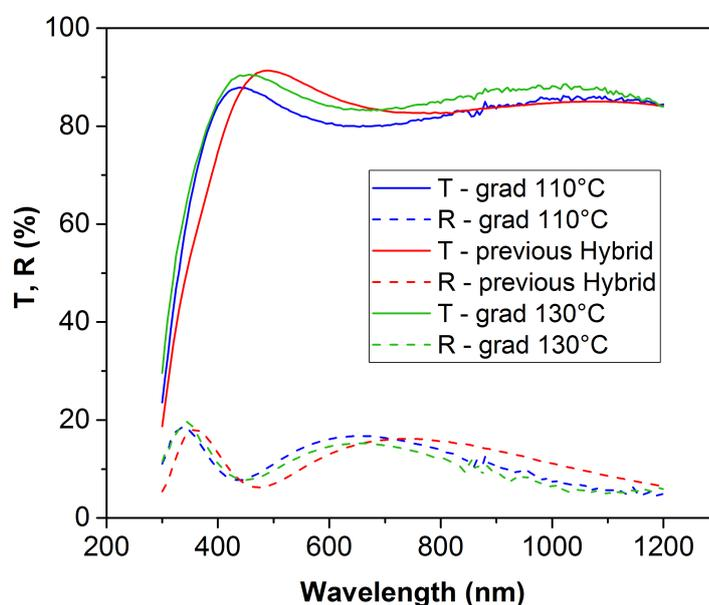
Figure 4.8: ITO transmittance and reflectance vs wavelength for different recipes.
