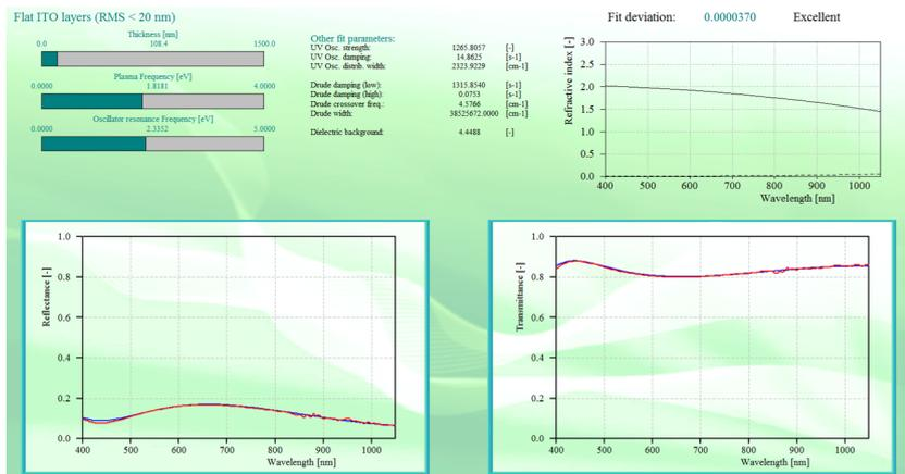
Figure 4.10: Fitting of transmittance and reflectance with existing models through SCOUT software.
