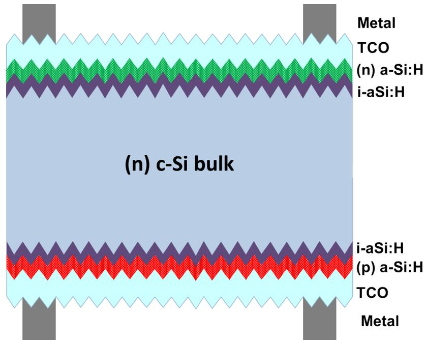
Figure 1.8: Structure of a Heterojunction with Intrinsic Thin Layer (HIT).
