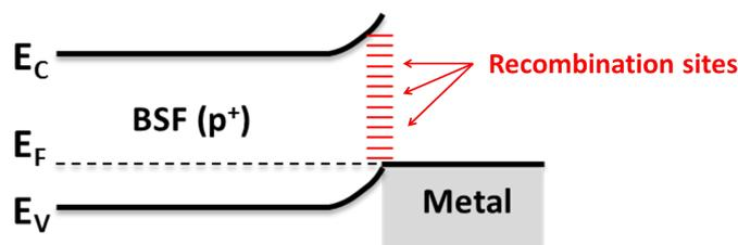
Figure 1.4: Contact recombination sites at the metal interface.
