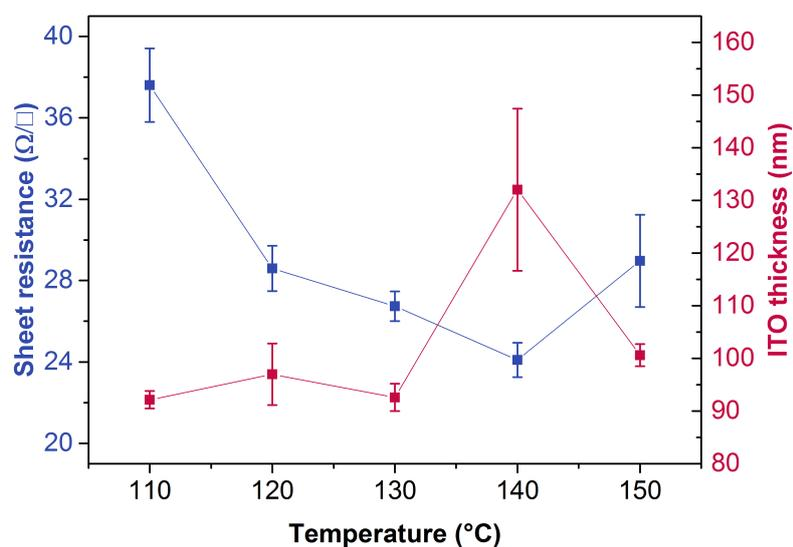
Figure 4.6: Sheet resistance and ITO thickness vs deposition temperature.
