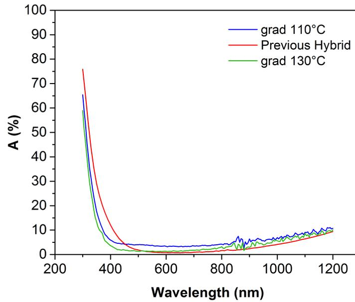
Figure 4.9: ITO absorbance vs wavelength for different recipes.
