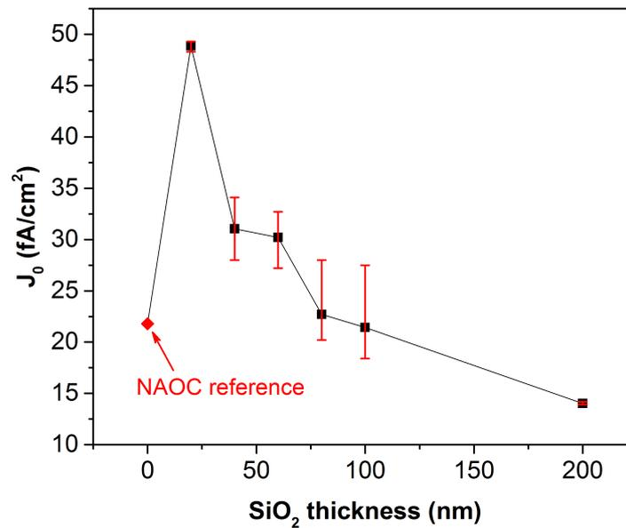
Figure 3.4:  $J_0$  vs oxide thickness.
