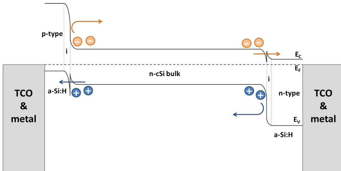
Figure 1.9: Band diagram of a HIT cell.
