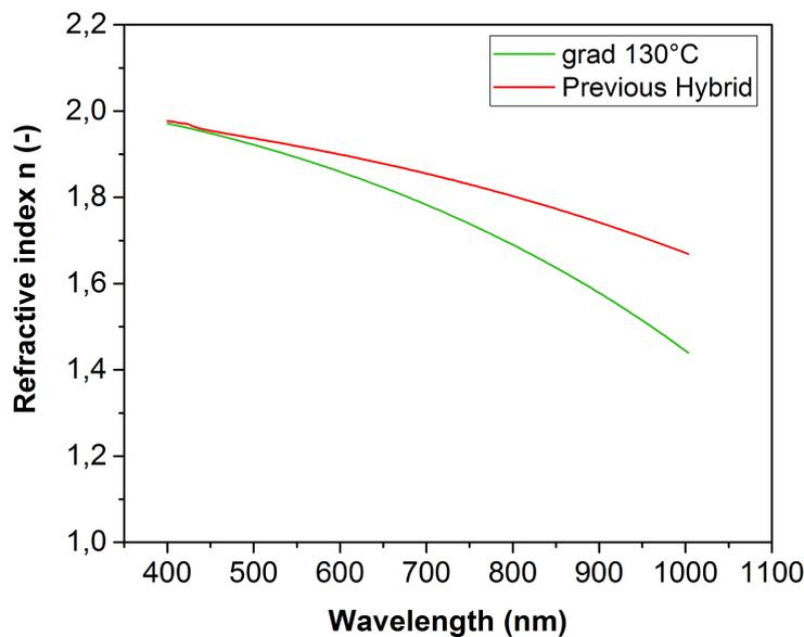
Figure 4.11: ITO refractive index  $n$  vs wavelength.
