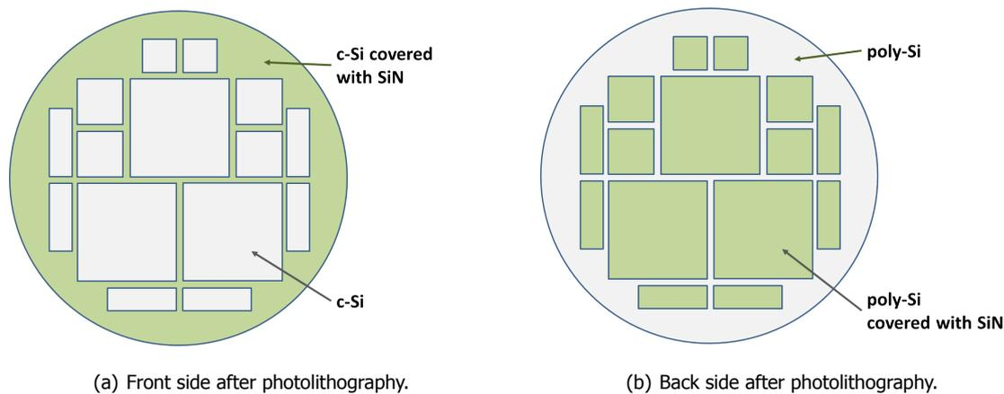
Figure 2.2: Front and back sides of a solar cell precursor before texturing.
