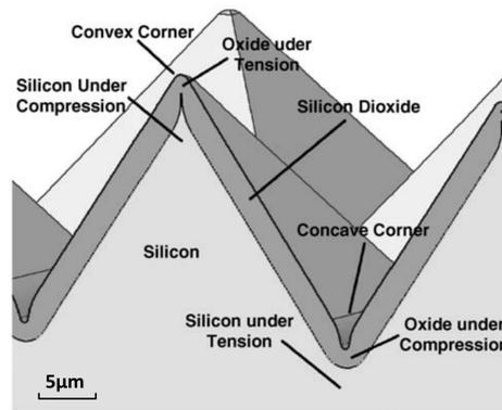
Figure 3.5: Schematic of an oxidized textured silicon surface illustrating the stresses induced [27].
