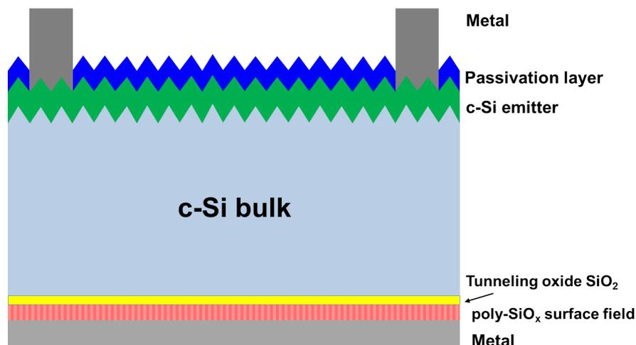
Figure 1.11: Structure of a silicon solar cell with a passivated rear contact.
