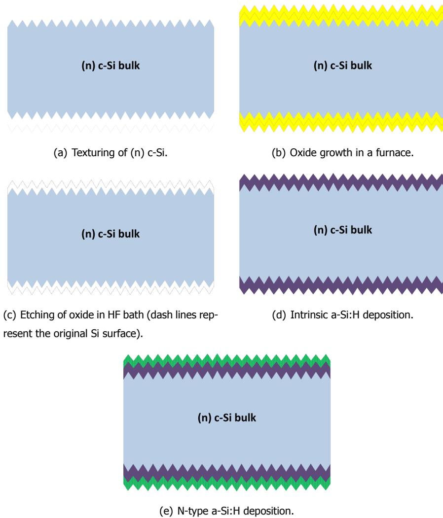
Figure 3.2: Flowchart for Thermal Oxidation Tests
