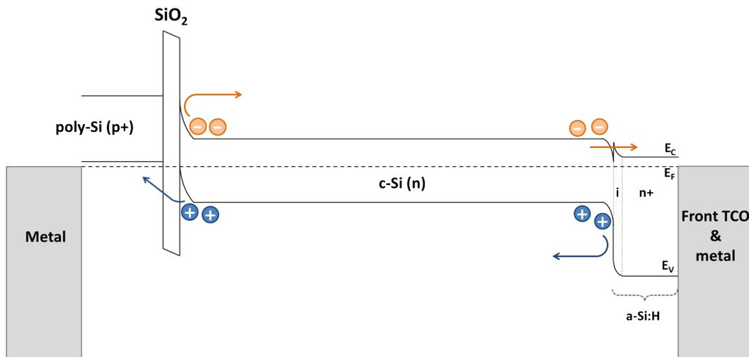
Figure 1.13: Band diagram of an Hybrid solar cell with poly-Si rear emitter.
