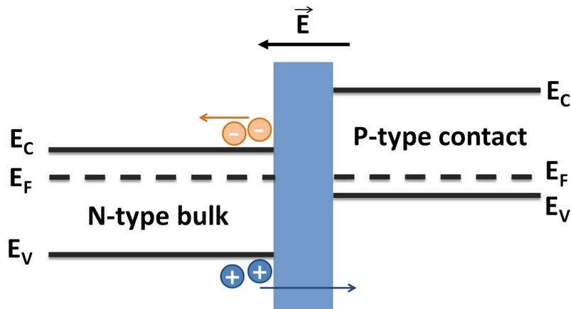
Figure 1.7: Schematic view of a field-effect passivation with an electric field  $\vec{E}$  introduced by the blue profile.
