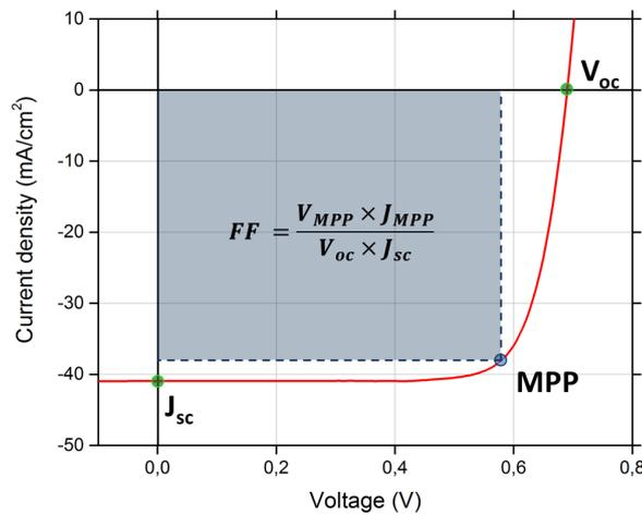
Figure 2.6: Typical JV-curve for a hybrid solar cell.
