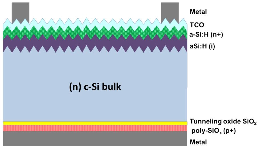
Figure 1.12: Structure of an Hybrid solar cell with poly-Si rear emitter.
