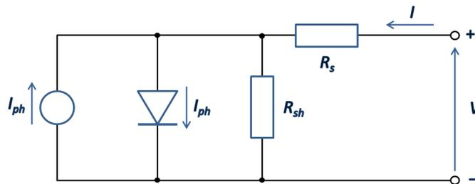
Figure 2.7: Equivalent circuit of a solar cell.
