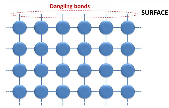
Figure 1.5: Crystalline silicon lattice with dangling bonds at the surface.
