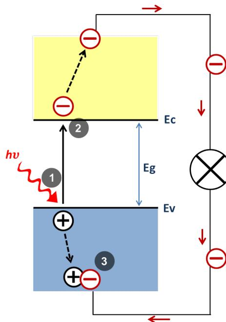
Figure 1.2: Principle of the photovoltaic effect: 1. Generation of charge carriers through the absorption of a photon ( $h\nu$ ). 2. Separation of the electron-hole pair. 3. Collection of the carriers through a circuit and recombination.
