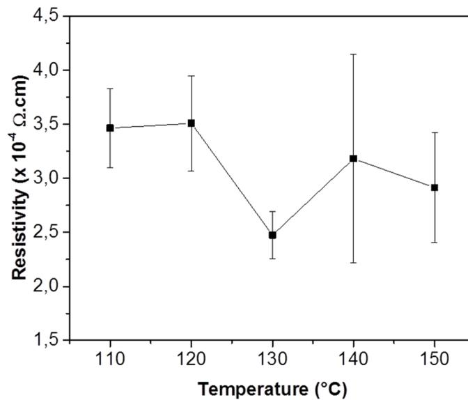
Figure 4.7: ITO resistivity vs deposition temperature.
