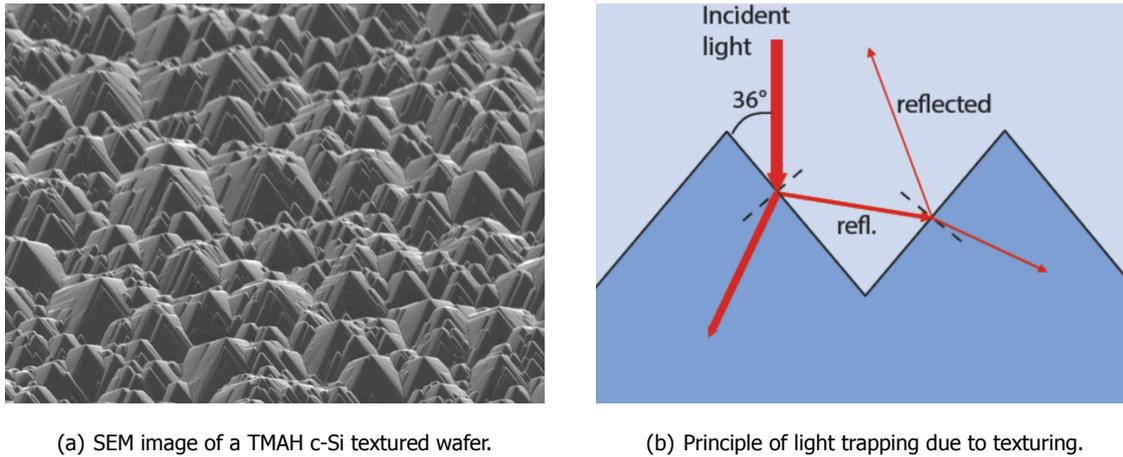
(a) SEM image of a TMAH c-Si textured wafer.
