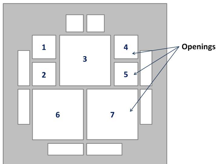
Figure 5.3: Hard mask for metal and ITO patterning.
