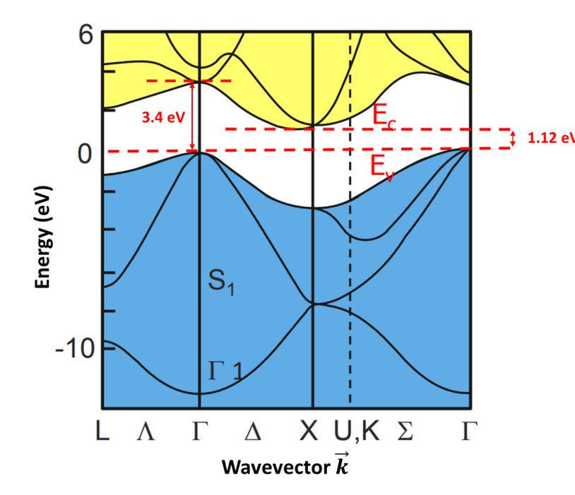
Figure 1.3: The band diagram of crystalline silicon [6].
