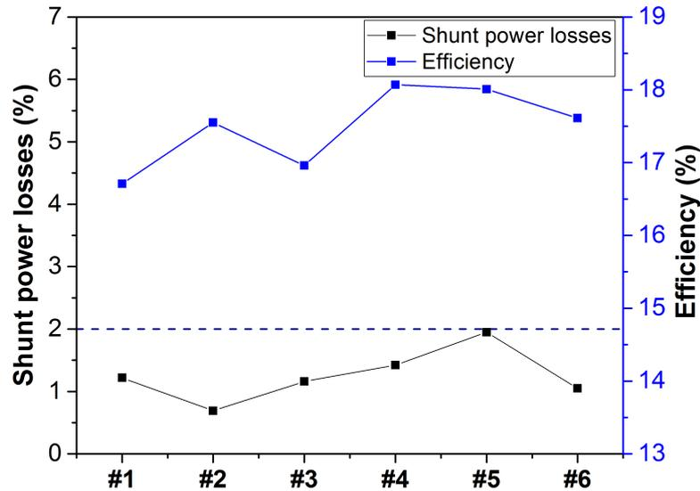
Figure 5.2: Global efficiency and power losses induced by a shunt effect for some Hybrid solar cells.
