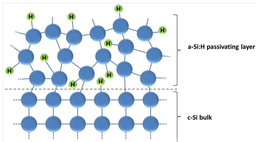
Figure 1.6: Crystalline silicon lattice with a passivating layer of a-Si:H at the surface.
