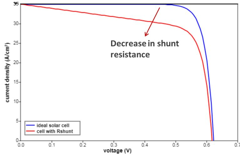
Figure 5.1: Effect of shunt resistance on JV curve [38].
