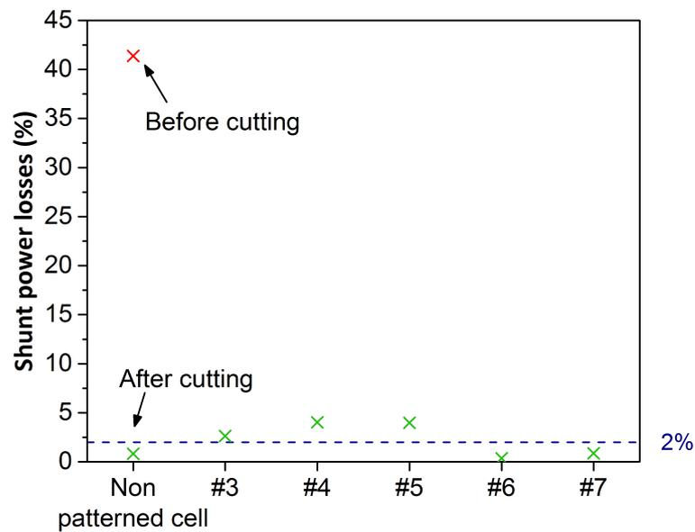
Figure 5.5: Power losses induced by the shunt resistance for different cells of a wafer, with patterned ITO and back metal.
