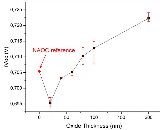
Figure B.1:  $i - V_{oc}$  vs oxide thickness.
