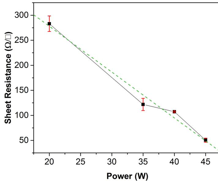
(b) Sheet resistance vs deposition power.
