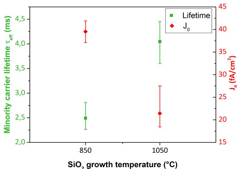
Figure 3.8:  $J_0$  and lifetime vs oxide thickness.
