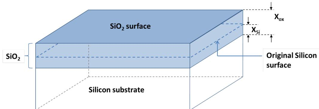
Figure 3.1: Thermal growth of  $\text{SiO}_2$  on top of Silicon.
