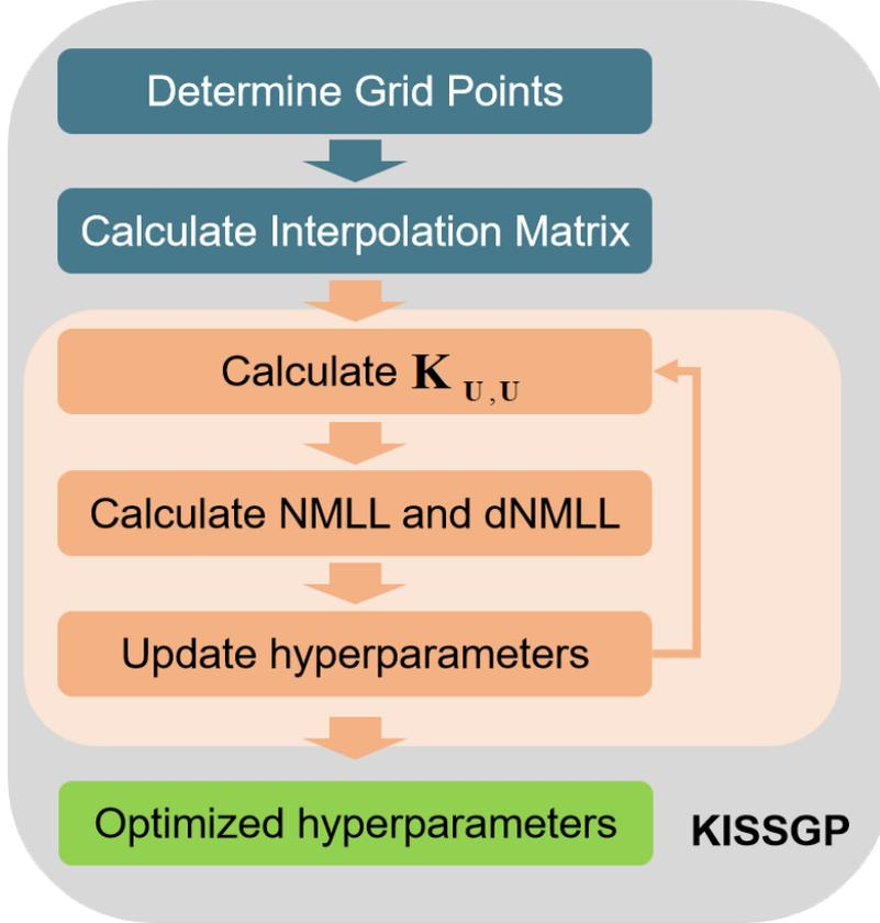
Figure 2.1: Training framework of KISSGP. The blue blocks represent the initialization phase, where the grid points and interpolation matrix  $\mathbf{W}$  are only calculated once. The orange blocks are the iterative steps in the algorithm, where the goal is to reach the lowest NMLL. The stopping criteria are set according to the nonlinear CG in algorithm 3, where the optimized hyperparameters are acquired
