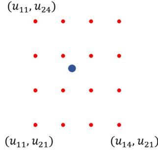
Figure 3.12: 2-D Interpolation Weights Calculation. The CCI for one point requires 4 grid points in 1 dimension. Thus 16 grid points in total are needed for 2-D.
