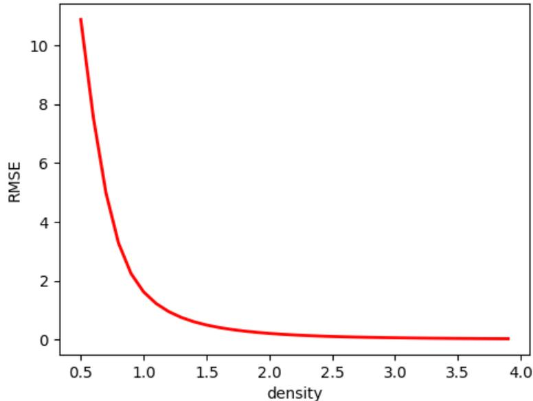
Figure 3.9: density vs. RMSE for RBF kernel reconstruction. When changing  $l$ ,  $d_u$ , and  $a$  with a fixed density, the RMSE value remains unchanged at the same relative positions. Thus this curve can be viewed as a theoretical curve for using CCI to interpolate an RBF kernel.
