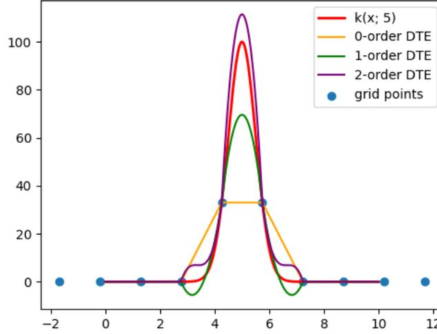
Figure 3.5: Interpolation results of different orders of DTE interpolation. The 1-order and 2-order DTE now generate a higher peak with error shrinking as the order increases. The 0-order DTE is equivalent to the linear interpolation.
