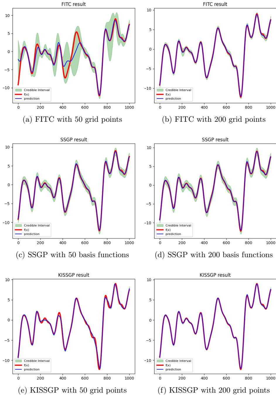
Figure 2.2: Comparison of the posterior distributions of different approximation methods. The first column contains the results with  $m = 50$ , whereas the second column contains the results with  $m = 200$ .
