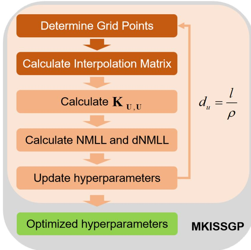
Figure 3.10: Training framework of MKISSGP. The two dark orange blocks were previously outside the optimization loop in the framework of KISSGP. Since the number of grid points is updated according to the length scale, these two steps should be recalculated at the beginning of every loop. The rest of the framework remains the same as in Figure 2.1.
