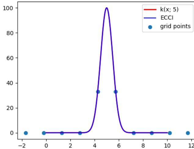
Figure 3.3: Interpolation results of ECCI. The interpolation and ground truth overlap because the RBF kernel is fully reconstructed by ECCI.
