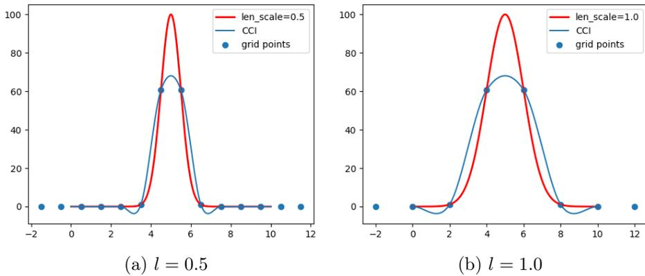
Figure 3.8: Comparison of interpolation result with  $\rho = 1$ . a) Using 16 grid points. b) Using 8 grid points. It can be observed that the red curves and blue curves are "stretched" along the  $x$ -axis.
