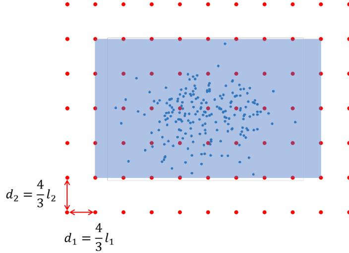
Figure 3.11: Example of a 2-D grid. The blue dots are the training points. The red dots are the 2-D grid points. The blue rectangle is the area that covers all training points. There is an additional padding of grid points around the blue rectangle so that the CCI is applicable at all training points.
