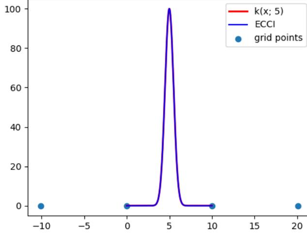
Figure 3.4: ECCI with only 4 grid points. In this plot, we reset the number and position of grid points so that all the interpolated points are within the center interval of the 4 grid points.
