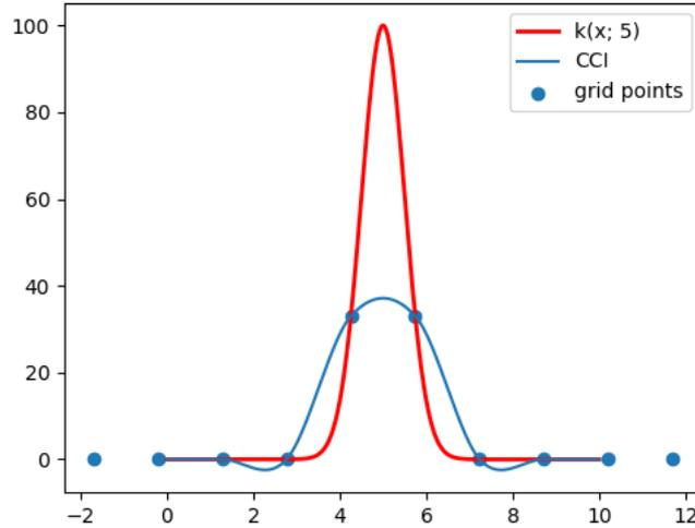
Figure 3.2: Interpolation results of CCI. The blue curve is the CCI which flattened the original peak due to the insufficient density of grids.
