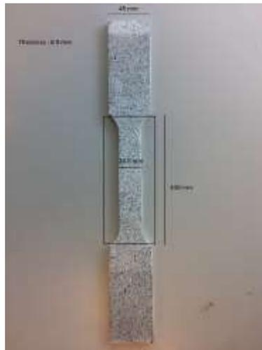
Figure 1. Dimension of the Steel Specimen
