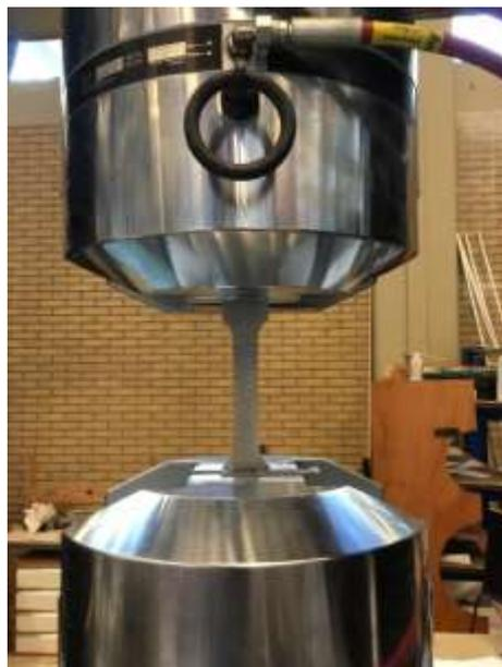
Figure 3. Tensile Test on The Steel Specimen
