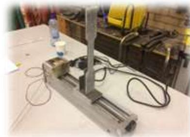
Figure 3. Calibration Machine and The Steel Specimen
