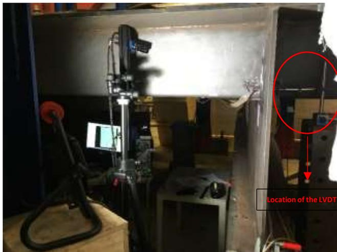
Figure 29. Location of the LVDT from side view
