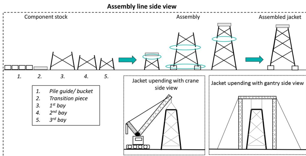
Figure C.1: Jackets assembly line
