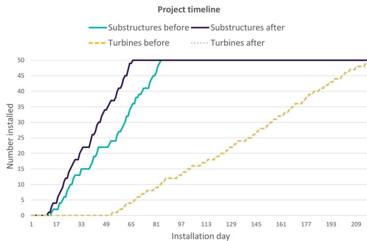
**Figure 5.22:** Project timeline for a "Single parameter change" study
