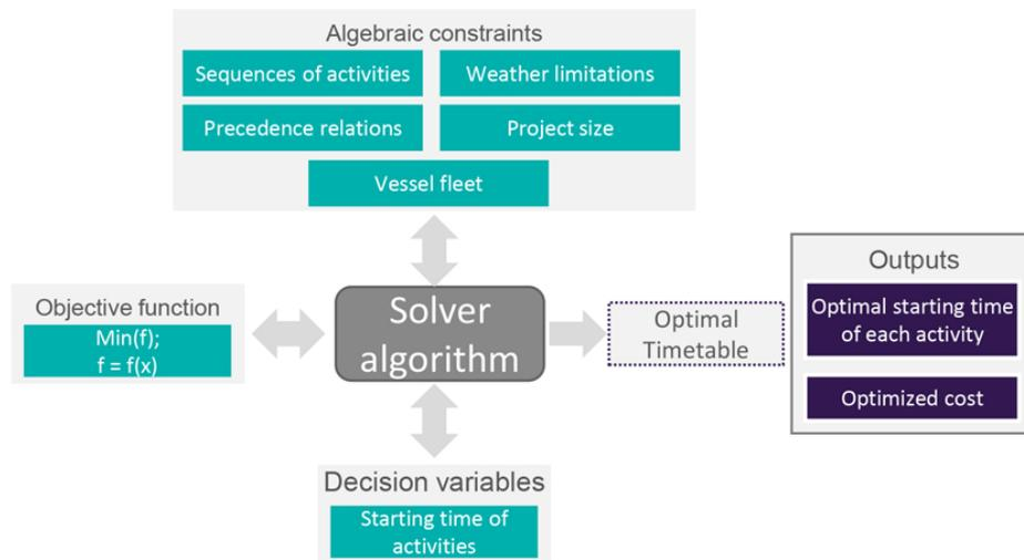
Figure 2.6: Generic structure of OWF installation optimization software
