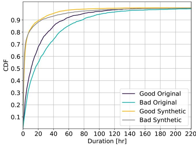
Figure 4.6: Good and Bad weather window CDF for original Markov Chain approach
