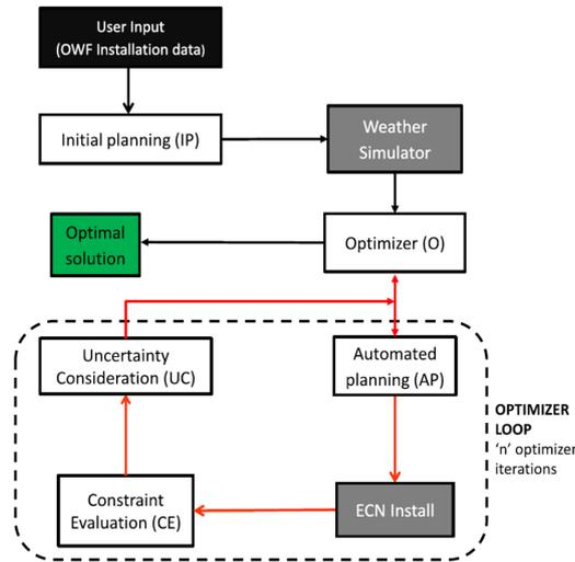
Figure 2.4: Upgraded ECN Install architecture (Kumar, 2017)
