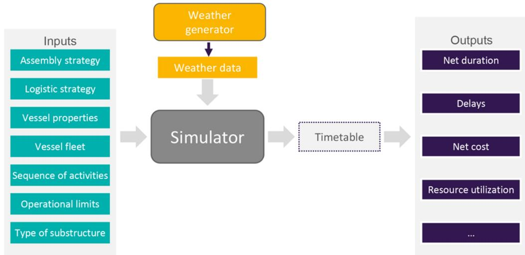
Figure 2.3: Generic structure of simulation-based OWF planner
