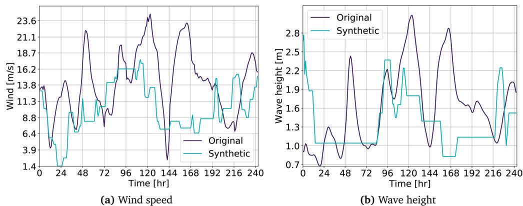
Figure 4.8: Zoomed weather series for adjusted Markov Chain approach
