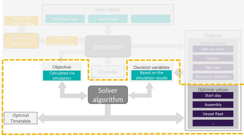
Figure 6.1: Optimizer diagram
