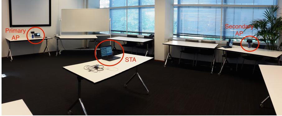
Figure 4.3: 60 GHz handoff measurement setup
