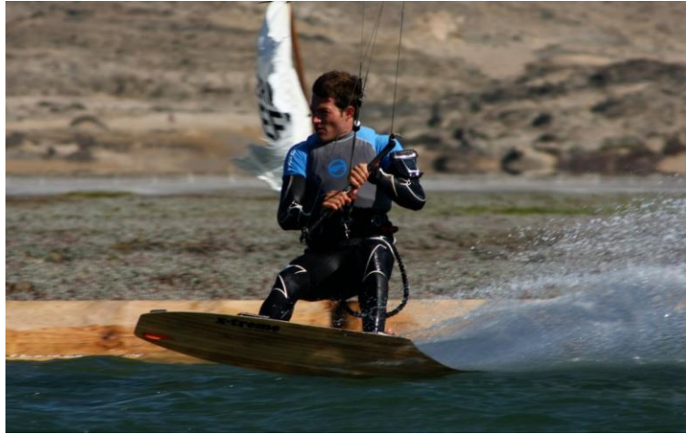
Figure 83, Looking at the bottom surface of the board during a speed run, it is clear that not the whole board is in contact with the water. Also next to the surface area that is below the water surface, there is an additional wetted area due to the spray above the surface. Picture: Graig Kolesky
