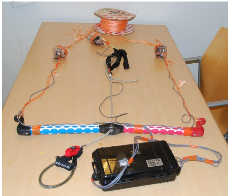
Figure 36, Picture of loadcell logger version 1. The principle of version 2 and 3 remained the same. Only the electronics where improved in subsequent versions.
