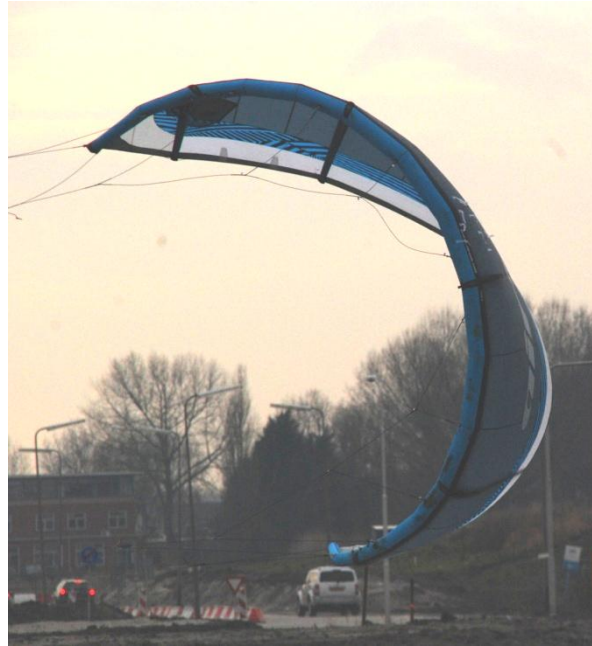
Figure 70, Extreme steering situation to illustrate the extreme spanwise variations in twist.
