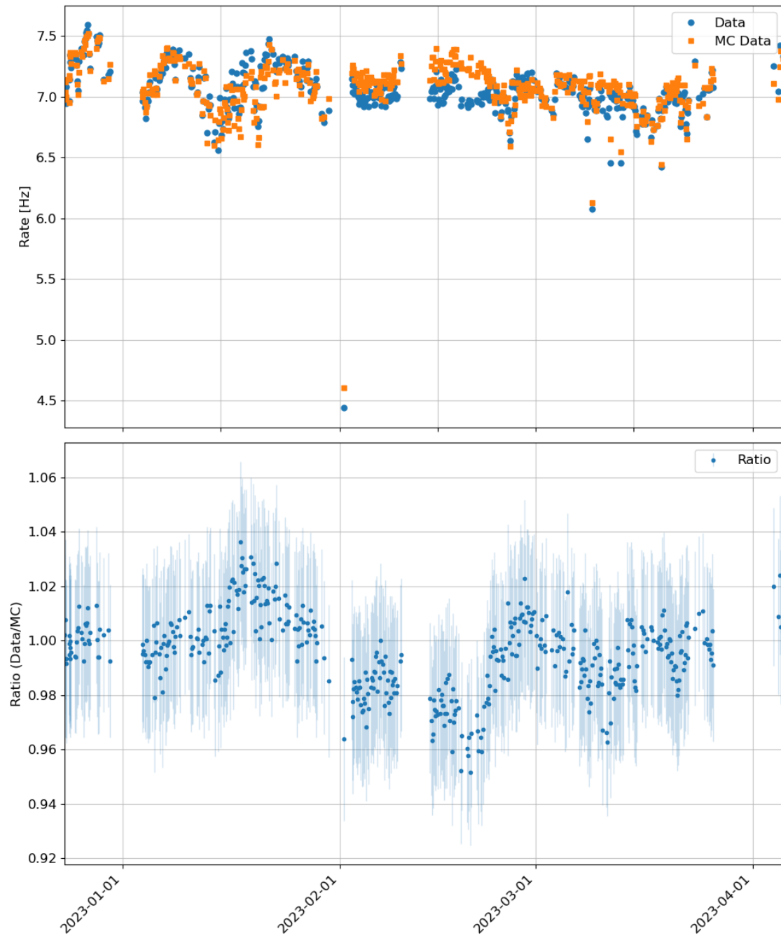
Figure A.4: Rate and ratio of data and the Monte Carlo simulation for ORCA-15 after cuts are applied. In the top part the count rates without error of the data and the Monte Carlo simulation are shown. In the bottom part the ratio of the two is shown with error.
