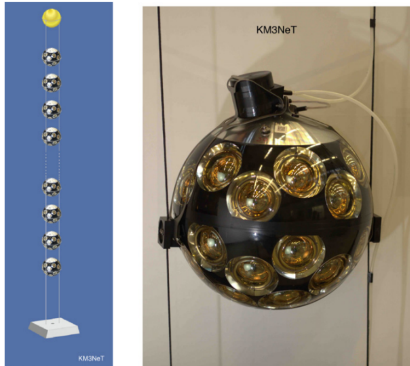
Figure 4.1: The detection unit (DU) left and the digital optical module (DOM) on the two thin parallel Dyneema ropes right [25].
