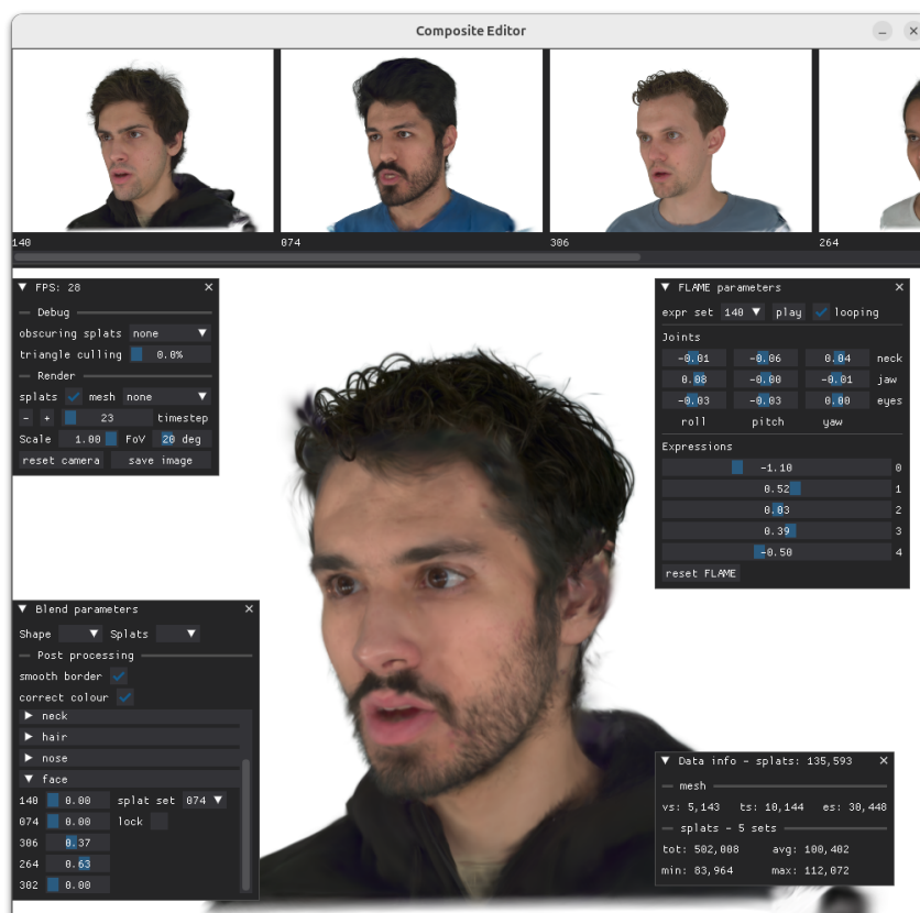
Figure 5.1: A screenshot of our editor. The bar on top displays a preview of the source avatars. The top left shows the debug panel, which can be used to toggle debug options such as changing the scale of the Gaussians or displaying the underlying mesh. The panel in the bottom left is used to edit the avatar by assigning Gaussians and modifying shape coefficients per region, as well as toggling the post-processing methods on/off. The bottom right panel displays information about the Gaussians and the mesh. Lastly, the panel in the top right is used to animate the avatar by selecting a set of expression parameters and iterating through them. It is also possible to manually adjust the joint parameters and the first 5 expression parameters.
