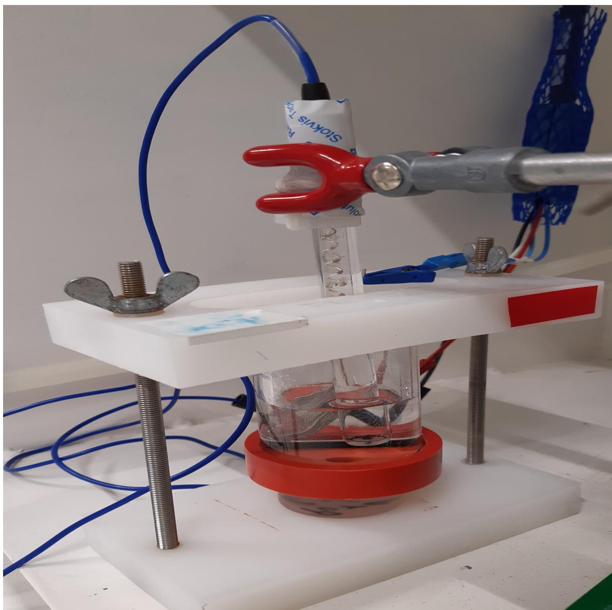
Figure A.2: Electrochemical cell used for CV and EIS measurement
