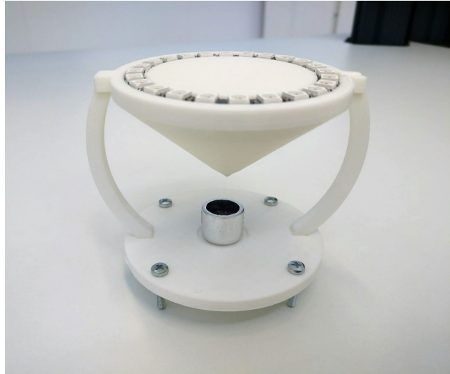
FIGURE 4.2: 3D printed proof of concept version of the antenna
