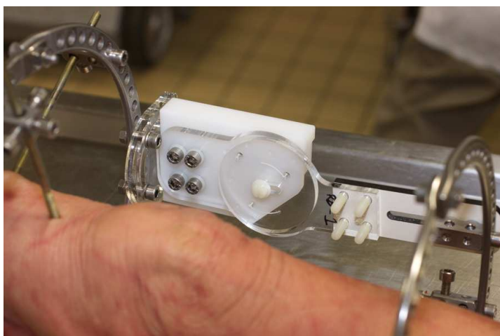
Figure VIII. Human cadaver knee used for evaluation of the movement reproduction principle.
