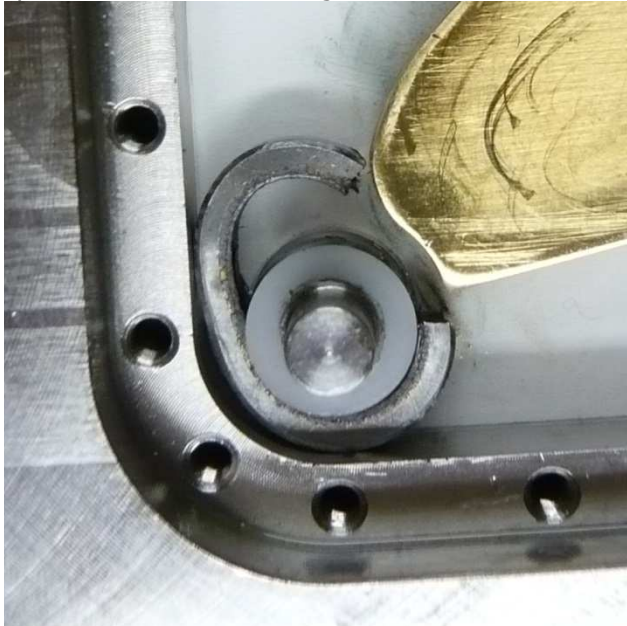
Figure X. Impression of the failed radial bearing. The motion prescribing part is positioned in the upper-right corner.
