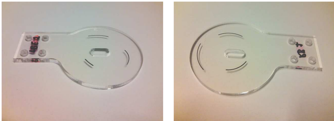
Figure VII. Registration plates resulting from measurements. (left: medial side of the joint, right: lateral side of the joint). The black lines show the recorded motion trajectories.
