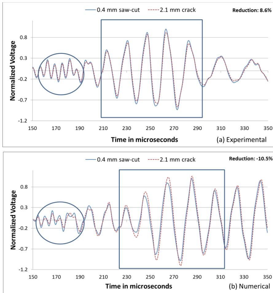
Figure 12: Model 1: Comparison of 50 kHz waveform between the 0.4 mm saw-cut versus the 0.4 mm saw-cut with 2.1 mm crack for Sensor 2.
