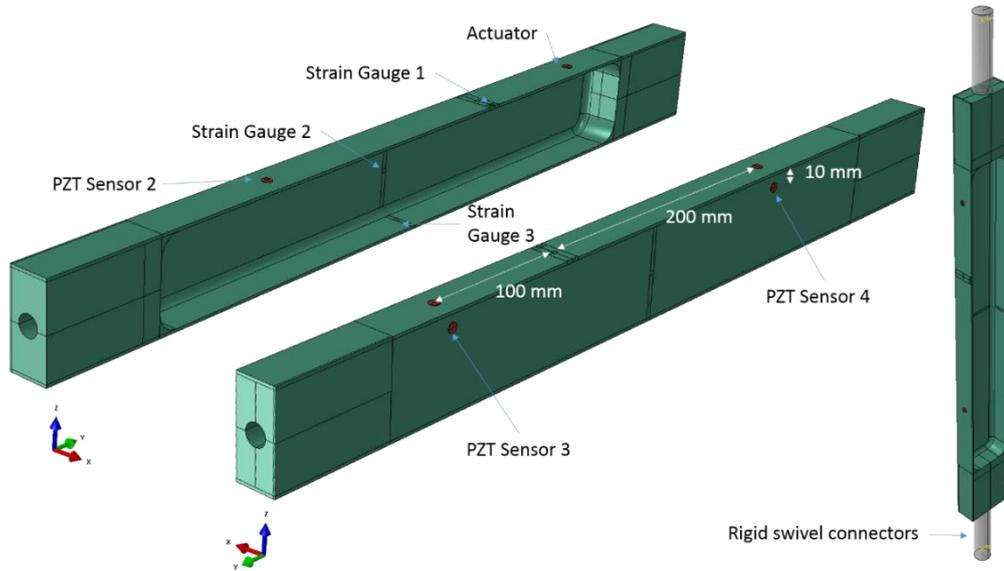
**Figure 3: Finite Element Model of the C-channel.**
