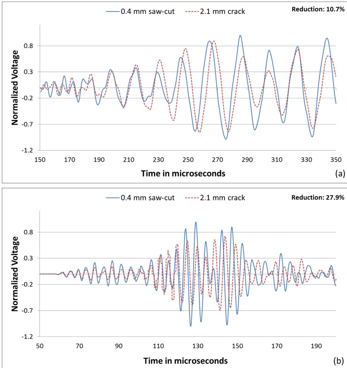
**Figure 18: (a) Model 3: Comparison of the 50 kHz waveform between the 0.4 mm saw-cut versus the 0.4 mm saw-cut with 2.1 mm fatigue crack for Sensor 2 with a residual stress field and an open crack; and (b) 200 kHz waveform.**
