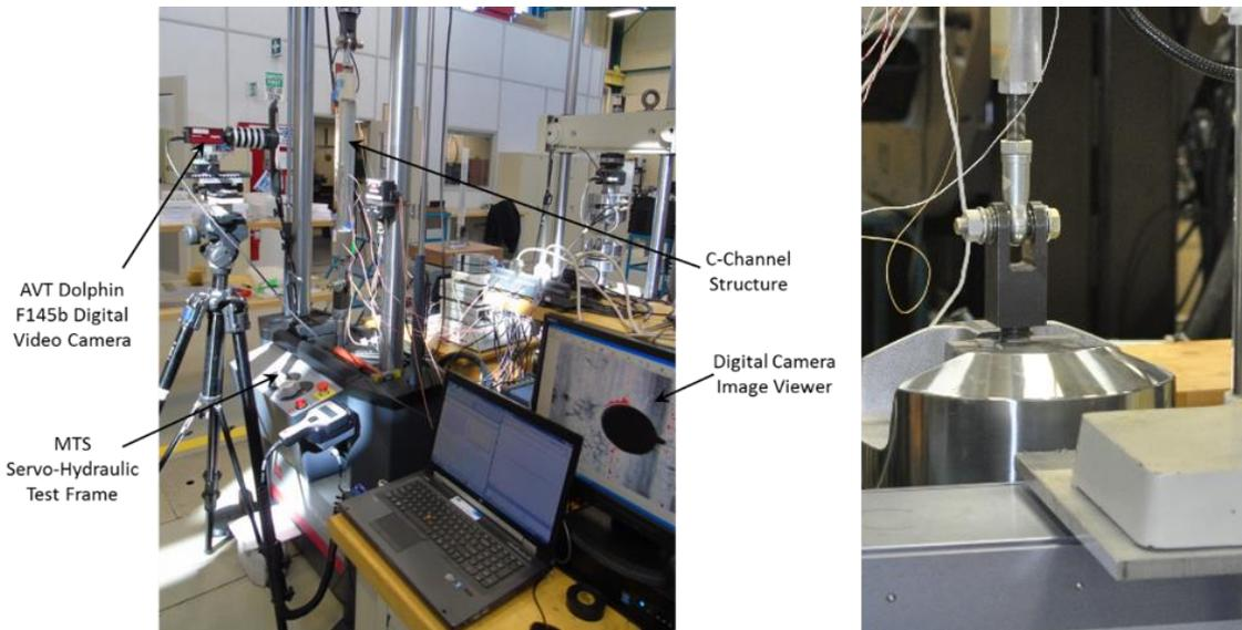
**Figure 2: a) Experimental setup; and b) Swivel loading condition.**
