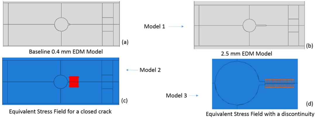
**Figure 6: FE Crack Growth Models: (a) Baseline FE Crack Growth Model with an initial 0.4 mm EDM notch and no residual stress field; (b) 2.5 mm EDM Model with no residual stress field; (c) 0.4 mm EDM under an applied internal load over a 2.1 mm region; and (d) 0.4 mm EDM + 2.1 mm 50  $\mu$ m width notch under an applied internal load.**
