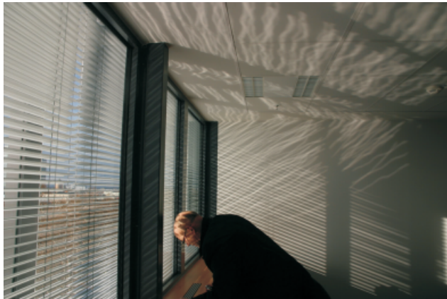
Figure 8. The Venetian blinds inside the cavity reflect daylight to the ceiling and thus deep into the room
