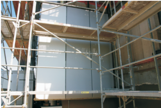
Figure 6. Mock-up of original façade panels with different new coatings: test of colour, reflectivity and weather resistance
