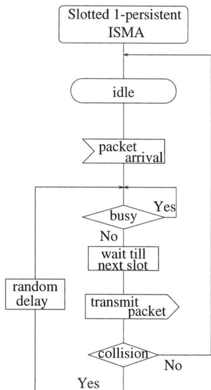
Figure 3.3: Terminal transmission of Slotted 1-persistent ISMA protocol.
