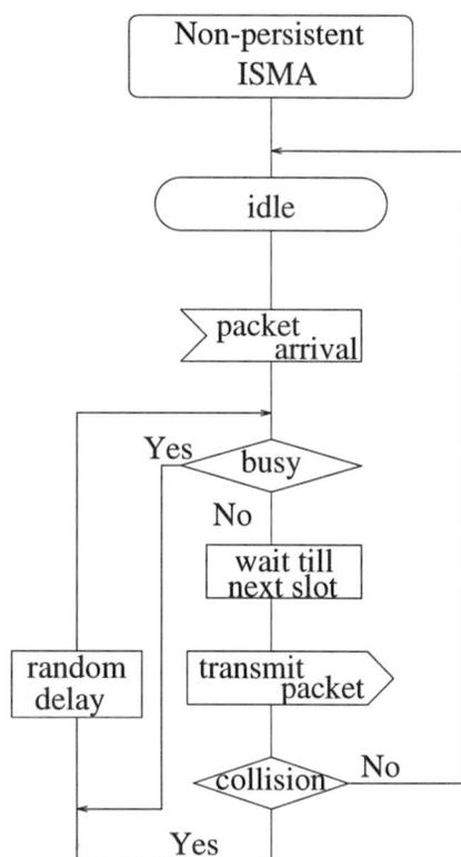
Figure 3.1: Terminal transmission of Slotted Non-persistent ISMA protocol.
