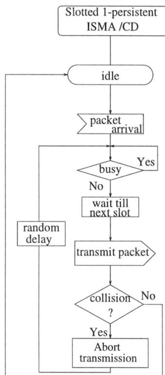
Figure 3.7: Terminal transmission of Slotted 1p-ISMA\CD
