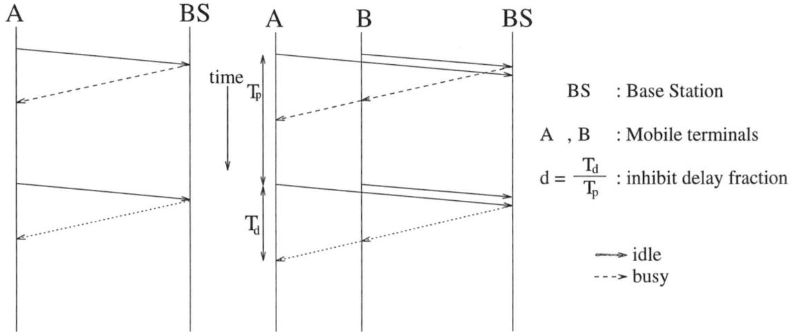
Figure 3.2: Slotted Non-persistent ISMA packet timing
