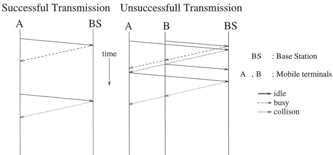
Figure 3.4: Collision Detection Timing
