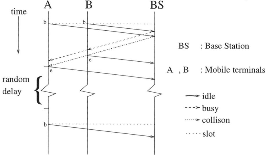
Figure 3.6: Slotted np-ISMA\CD Packet Timing
