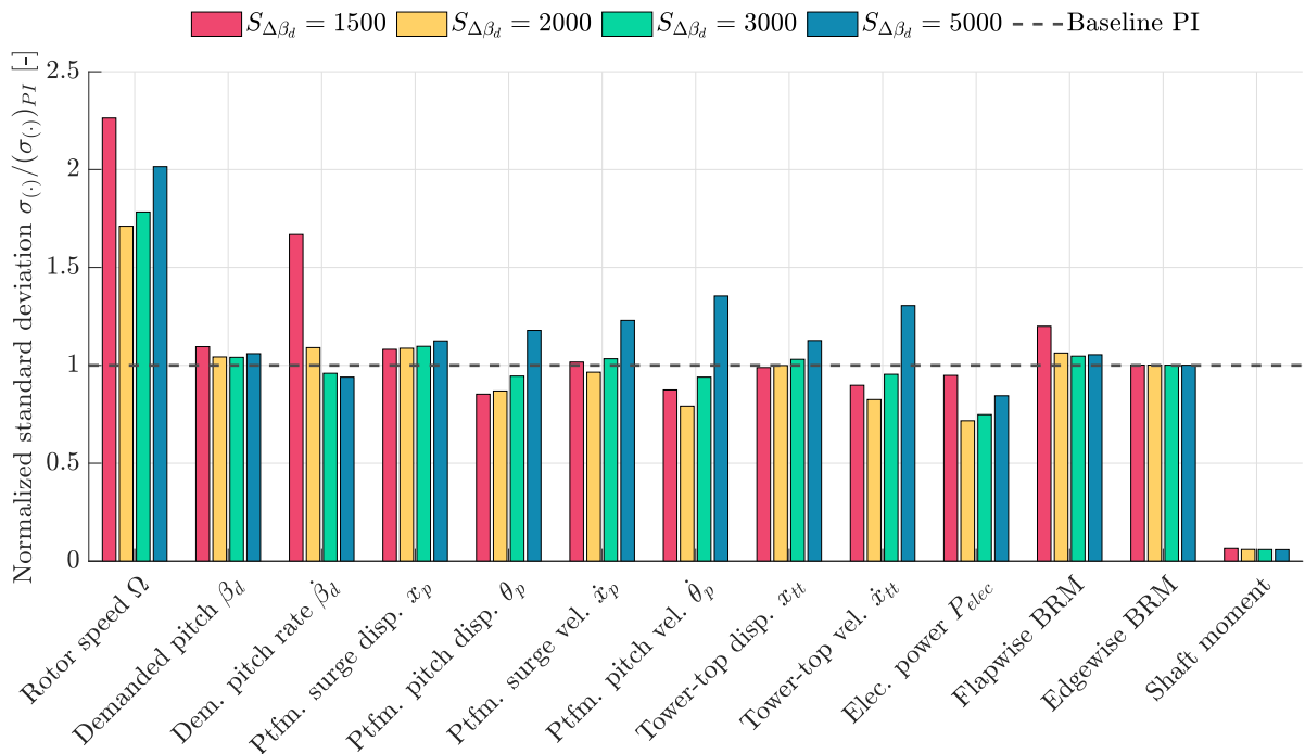
Figure 5.22: Tuning of blade pitch rate penalty S_{\Delta\beta_d} , under turbulent wind simulation, with average wind speed 14 m/s and 10% TI. The normalised standard deviation of relevant signals are shown for several weighting values. The weight for platform pitch motion minimisation is W_{\dot{\theta}_p} = 500 , and the weight for rotor speed tracking is W_{\Omega} = 20 , for all cases.
